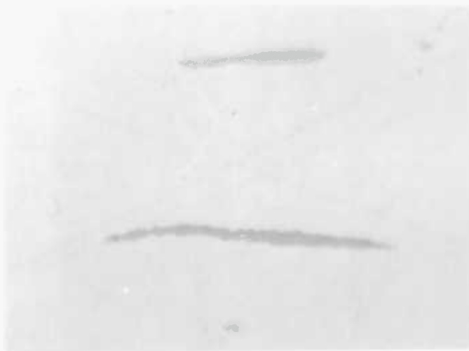
Plate 5.1 Inclusions in En 32B, x 1900
