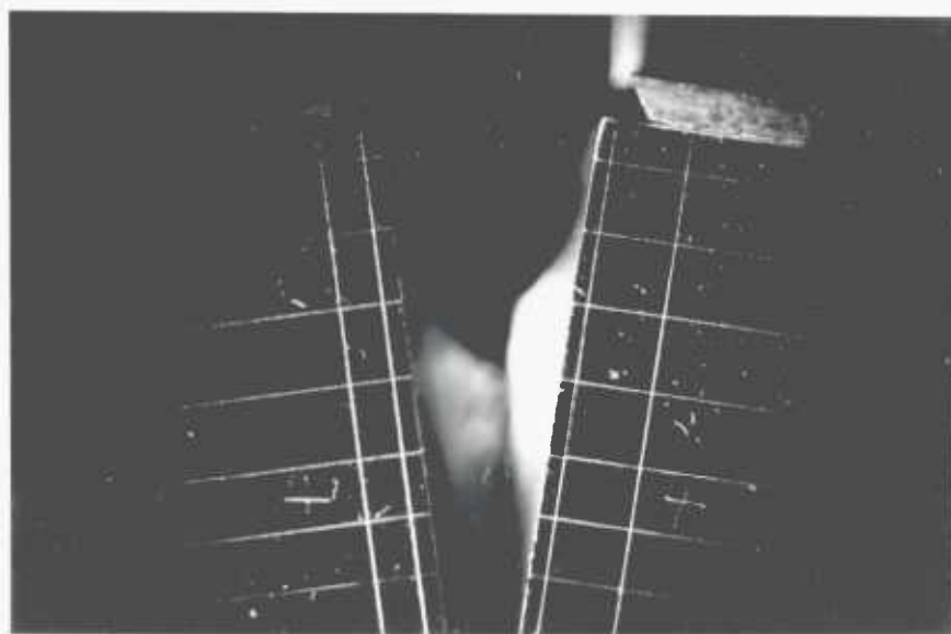
Plate 9.2. Grids on surface of bend specimens of En 32B, used for deriving rotational factors.
