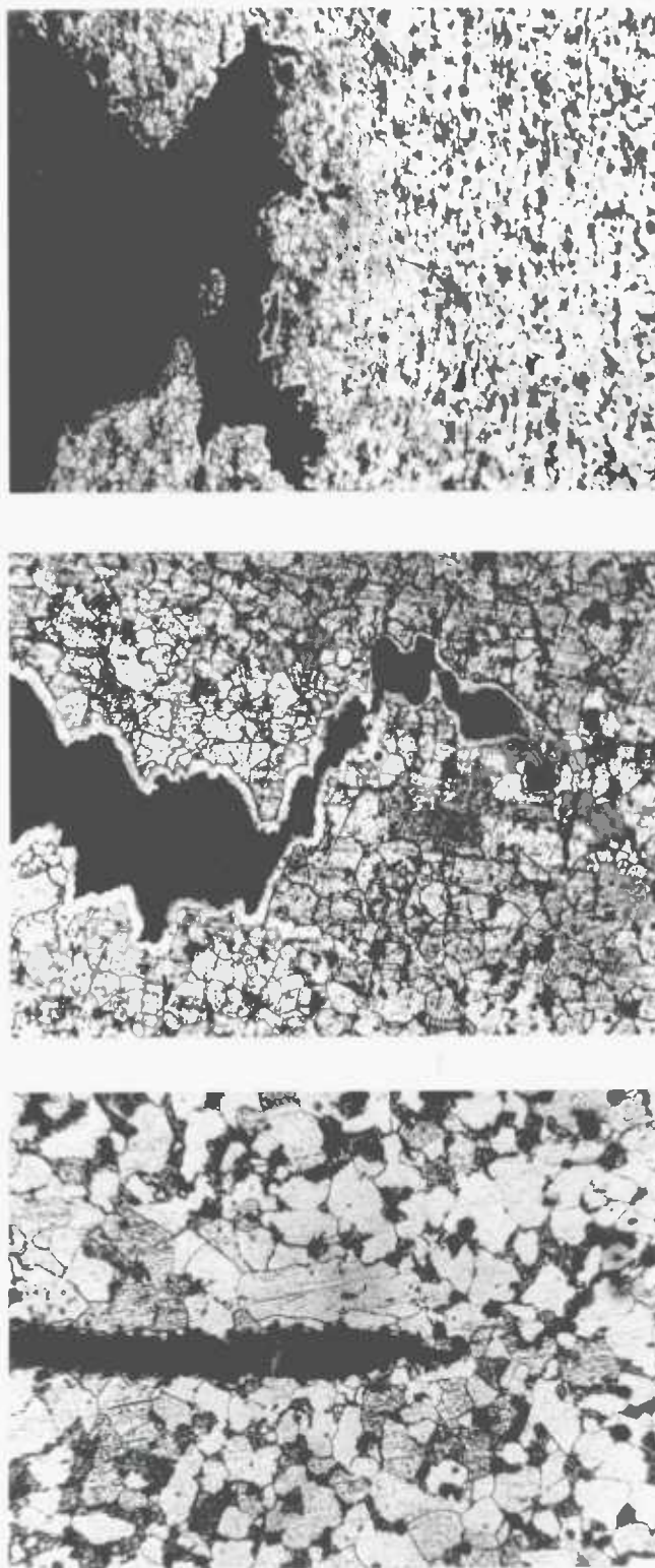
Plate 8.1. Crack tip profiles in En 32B, recrystallised, etched nital.
