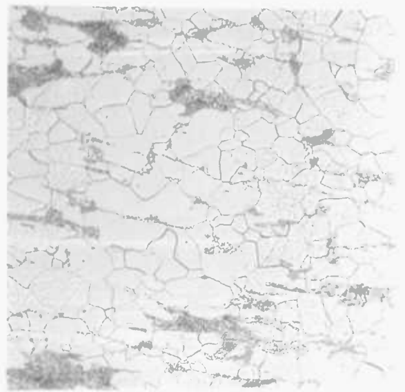
Plate 5.7 Recrystallised grains in En 32B, etched nital, x 500
