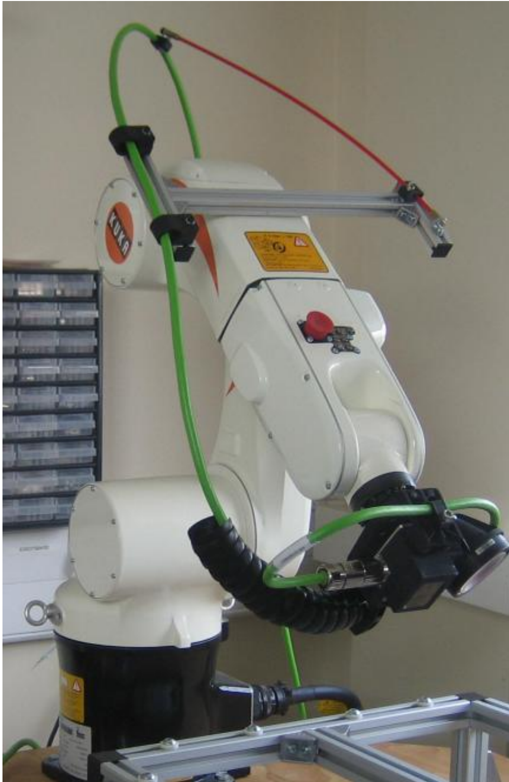
Figure 4.16 The LSA Robot Scanner, an ILS2100 integrated with an industrial pick-and-place robot and custom control software.
