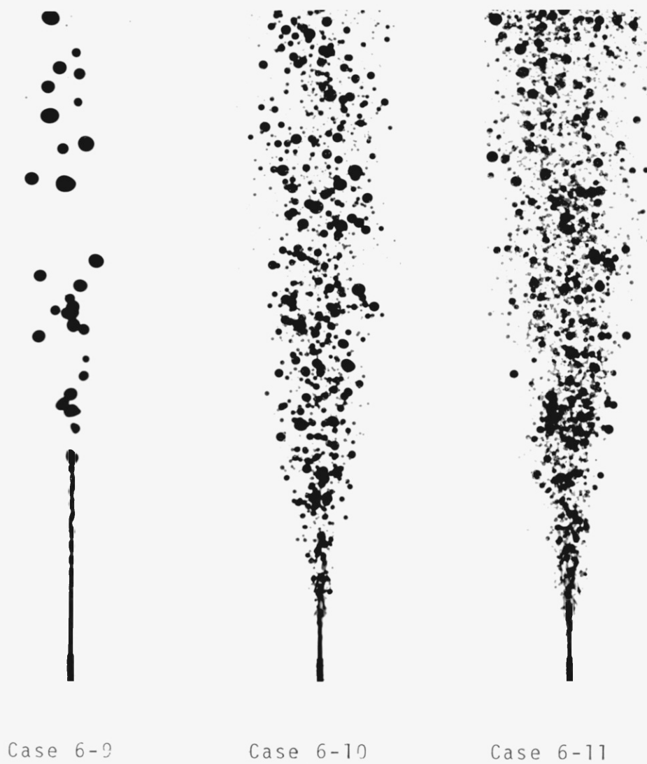
Fig. 6.44-1 Overall views of kerosene-into-water steady jet: Cases 6-9, 6-10, 6-11
