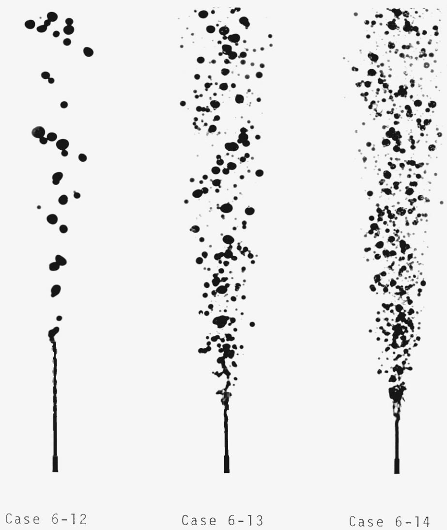
Fig. 6.44-2 Overall views of kerosene-into-water steady jet: Cases 6-12, 13, 14
