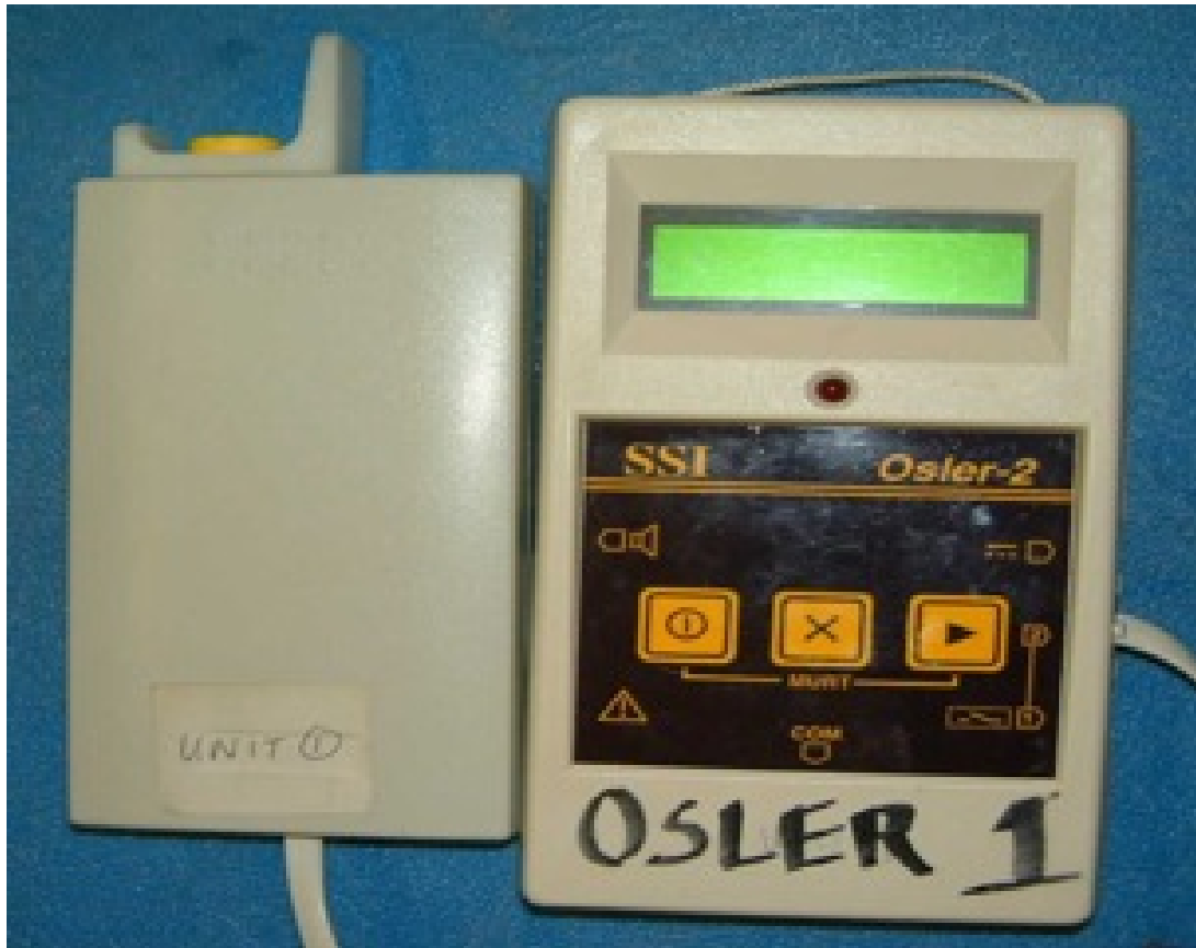
Figure 2.6: The OSLER test equipment (Stowood Scientific Instruments, Oxford, UK)
