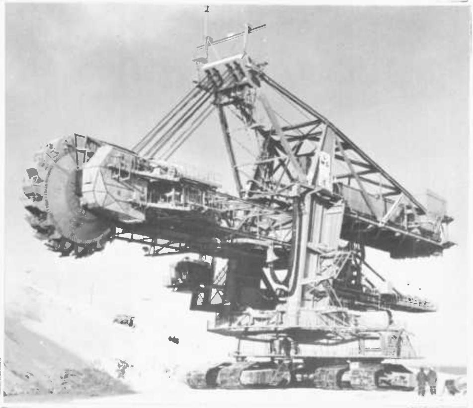
FIG.20a BWE FOR HARD GROUND OPERATION, ATHABASCA TAR SANDS
