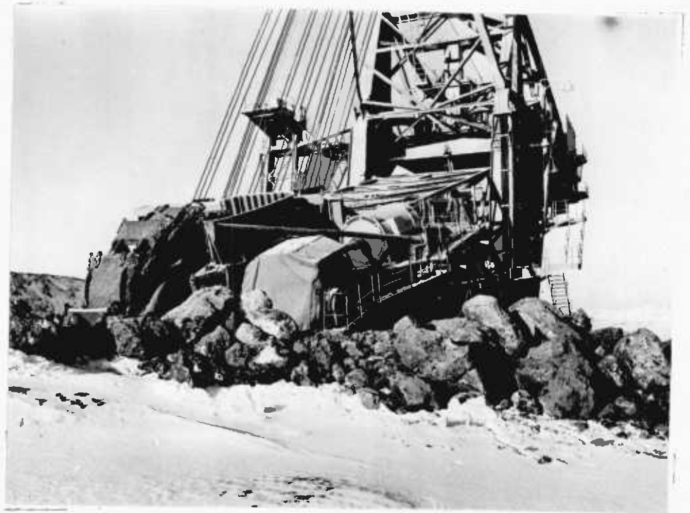
FIG.20b BWE HANDLING LARGE LUMPS IN HARD GROUND, ATHABASCA
