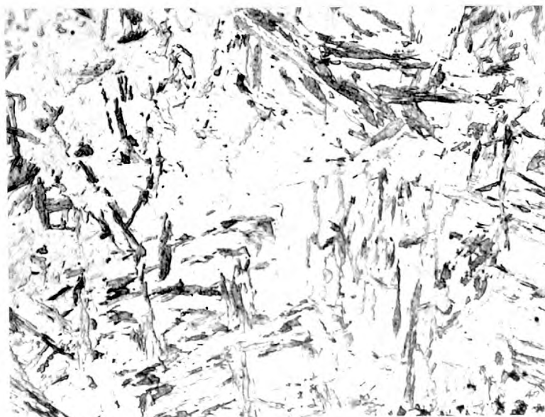
FIG. 22. THE MARTENSITE PLATES FORMED ON COOLING 8°C BELOW M_s , AFTER AUSTENITIZING AT 750°C.
