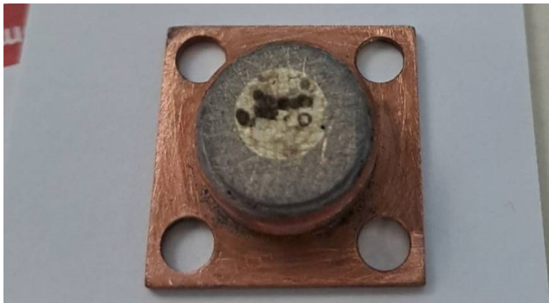
Figure 3.3: A photo of a used target. There are several holes drilled by YAG laser, and a layer of coating can be seen clearly.
