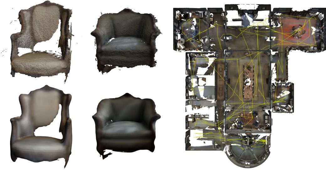
Figure 5.1: Objects reconstructed using our method [Top left] and their corresponding ground-truth meshes provided by the Matterport3D dataset [Chang et al., 2017] [Bottom left]. Top-down view of 3D reconstruction after exploration, and MAV path in yellow [Right].
