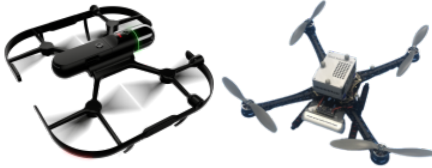
Figure 6.7: MAVs used for real-world experiments. [Left] Leica BLK2Fly with LiDAR. [Right] Custom MAV with Intel RealSense D455 RGB-D camera.
