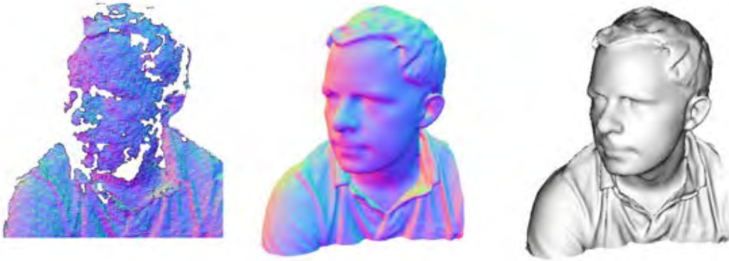
Figure 2.3: Input point cloud [Left], surface reconstruction normals [Middle] and Phong-shaded surface reconstruction [Right] using KinectFusion . Images from [Newcombe et al., 2011].
