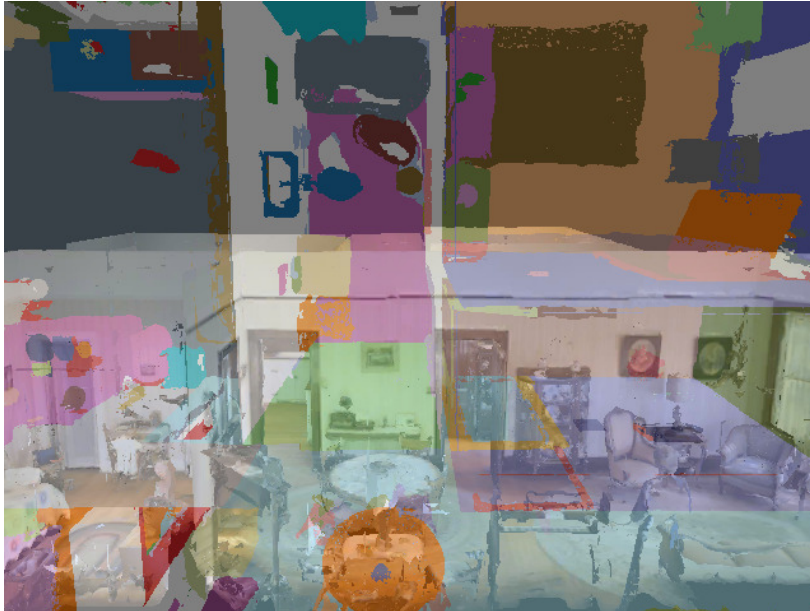
Figure A.3: Modern Architecture (2022): Visualisation of the ground-truth colour and instance ID meshes from the 2t7WUuJeko7 scene of the Matterport3D dataset [Chang et al., 2017]. A prime example of the most common issue in robotics, a transformation being wrong.
