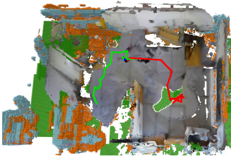
Figure 2.11: Example of semantic scene completion in SC-Explorer . Top-down view of the TSDF reconstruction with predicted voxels in orange, cyan, and green. The goal path shown in green is towards a region with high completion uncertainty. Image from [Schmid et al., 2022].
