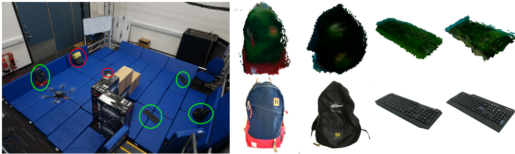
Figure 5.9: [Left] The real world experimental setup and the MAV. Detected and undetected objects are circled in green and red respectively. [Top right] Meshes of the 2 backpacks and 2 keyboards reconstructed during the experiment. [Bottom right] Photos of the corresponding real world objects.
