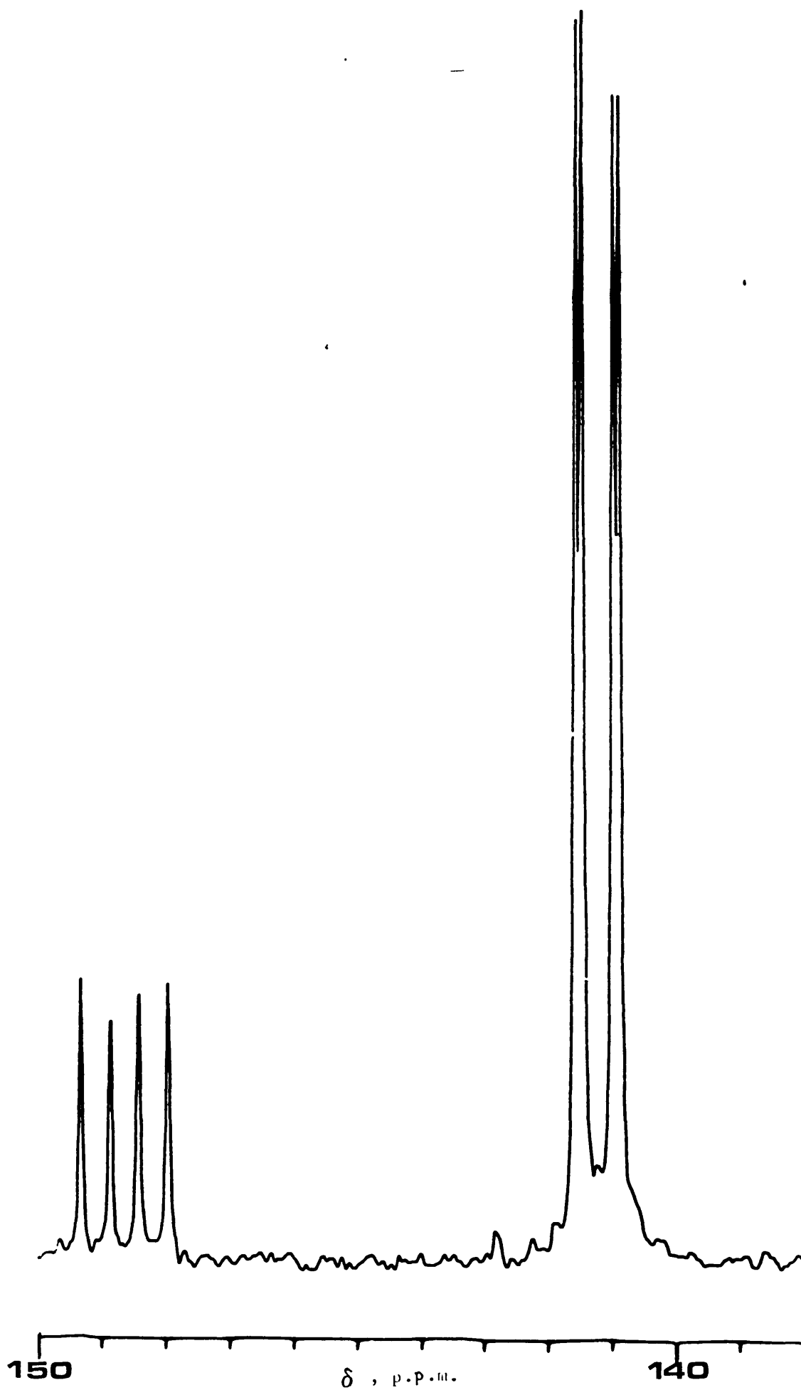
Fig 2.5 ^{13}\text{C} n.m.r. Spectrum of [\text{RhH}(\text{CN})_5]^{3-}
