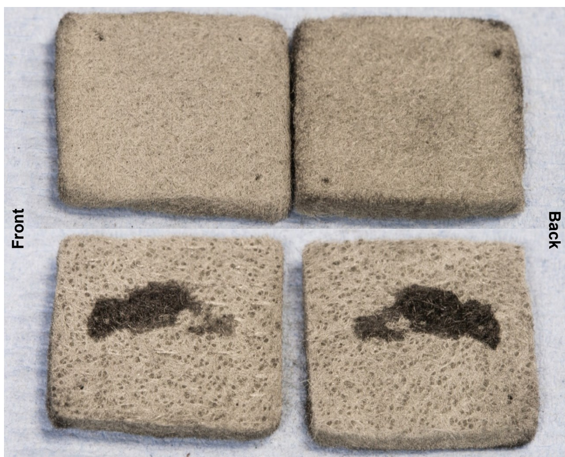
Figure 7-5: Images of outside (top) and inside (bottom) of plated felt achieved at -1.4 V (AgCl|Ag) for 2 hours in aqueous solution containing 0.3 M SnCl 4 and 2.2 M KOH flowing at 132 ml min -1
