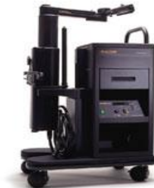
Figure 2.5: The AESOP voice controlled laparoscope positioning system which was the first FDA approved robotic device to be routinely used within operating theatres. The system held the laparoscope and provided the surgeon with a stable field of view and reduced the number of operators required in the operating theatre. Image source: Computer Motion Inc.
