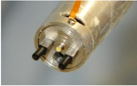
Figure A.7: The twin Medigus IntroSpico™ cameras can be clearly seen protruding from the tip of the robot. The cameras have a baseline of 5mm and a vergence of 0.5°. The light source can also be seen between the two cameras
