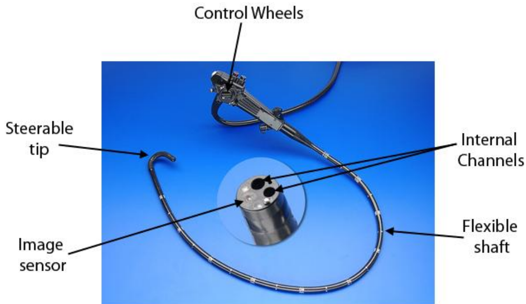
Figure 2.8: A dual-channel videogastroscope with the steerable tip, control wheels, image sensor, two internal channels and flexible shaft highlighted. Image source: Karl Storz Endoskope GmbH.
