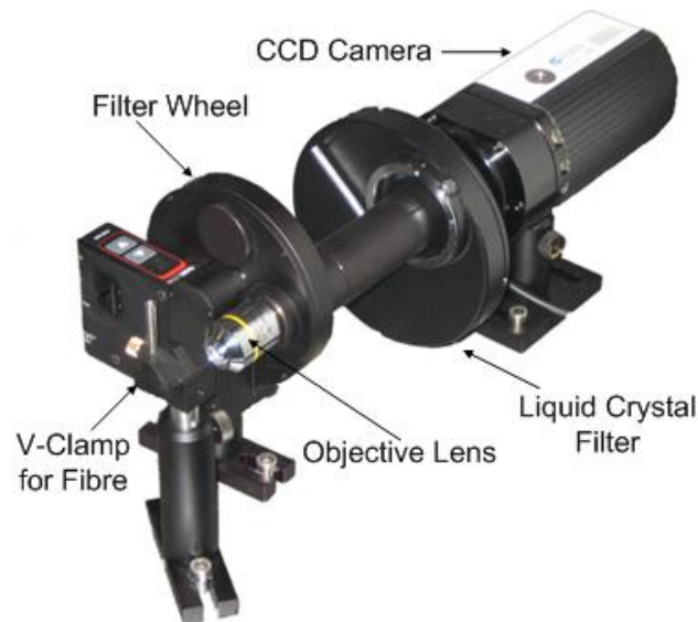
Figure 3.4: Image acquisition system used with the multi-spectral imaging robot including fibre clamp, liquid crystal tunable filter and CCD camera.
