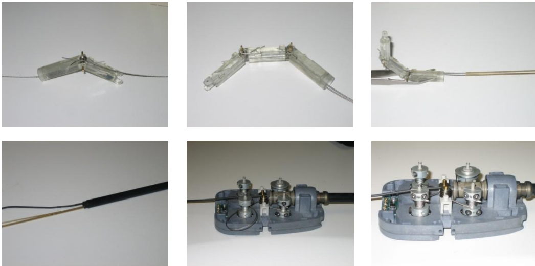
Figure A.1: Six images showing several of the steps required to wire and pretension the articulated segment of the robotic probe. (1,1) The base joint showing the connection to the rigid shaft and the first link. The legs of the torsion spring, the axle and the tendon are also visible. (1,2) shows two joints with three links connected. The effect of embedding the torsion spring with 120^\circ between the legs is evident as the joint assumes an inverted orientation since there is no tension in the tendons to act against the springs. (1,3) shows the tendons running out of the articulated segment with the brass rods clearly visible. (2,1) The brass rods running into the rigid shaft can be clearly seen as well as a hollow rubber tube used to protect the fibre bundle. (2,2) The capstan configuration can be seen here, with the front left capstan unwired and the front right capstan wired. (2,3) the final tensioned configuration. The protective tubing for the fibre bundle can also be clearly seen exiting the shaft
