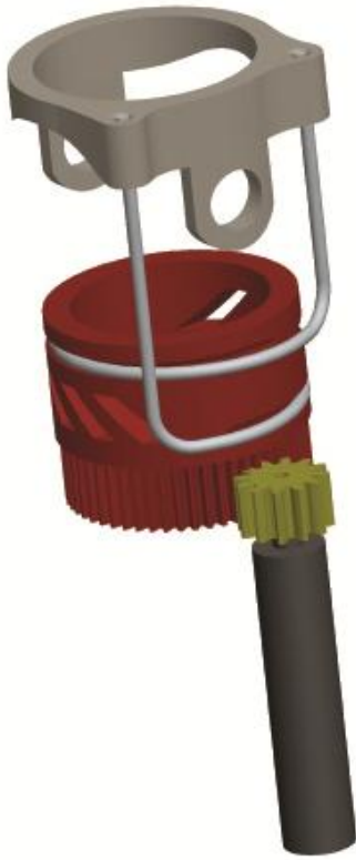
Figure 4.2: CAD schematic illustrating the key elements of the conceptual design utilising the hybrid micromotor-tendon actuation scheme.
