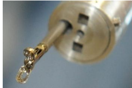
Figure A.8: The internal channel can also be used to pass endoscopic instrumentation, such as a biopsy forceps
