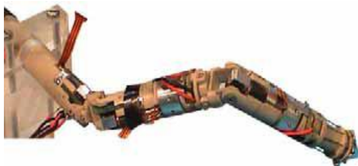
Figure 2.10: Dexterous Robotic Arm for Cardiac Artery Bypass Grafting. The system features embedded actuation which offers significant advantages for reducing the footprint in-theatre, however the design does not provide any space for internal channels to pass instruments or control wires. Image Source: [88]
