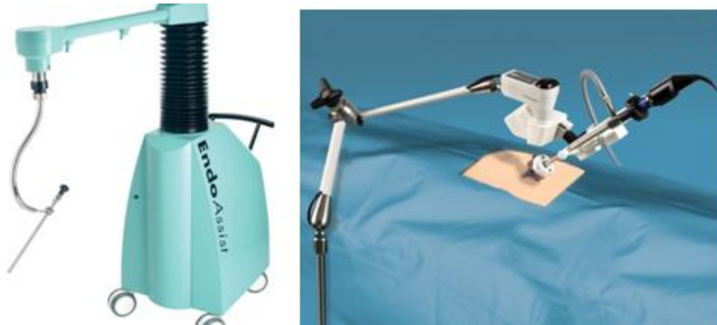
Figure 2.6: The EndoAssist (left) and Freehand Surgeon (right) laparoscope positioning systems which use a surgeon mounted IR tracker to control the laparoscope field of view. Image source: Prosurgics Inc.
