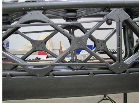
Figure 2-11: The internal structure of a Wellington Bomber whilst being reskinned at RAF Museum Cosford. Small holes used for pinning the fabric in place are visible in the structure
