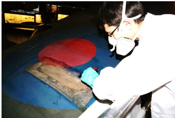
Figure 3-8: The process of applying a dope-fabric patch to a tear in the Hawker Hurricane on display in Flight . Top left to right; a tear in the Hawker Hurricane; working at height to fit a linen patch to the tear area; applying dope to secure the patch in place; the tear seen from the walkway after in painting (images ©Richard Horton/The Board of Trustees of the Science Museum, London)
