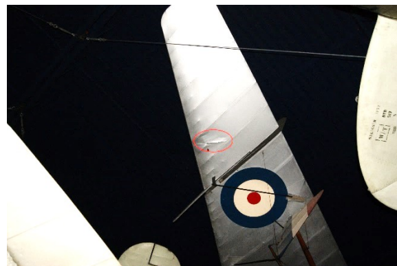
Figure 3-5: Tears in the doped-fabric skins of the JAP Harding Monoplane (left) and the Pterodactyl (right) lying well beyond human interference
