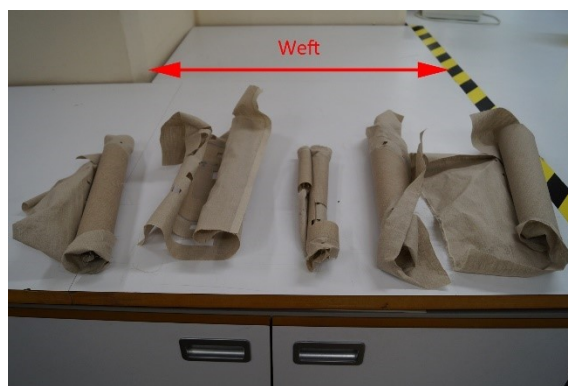
Figure 8-1: Doped-fabric panels of 9F1 Irish Linen treated with 9701 Randolph Butyrate dope after removal from the acrylic frame
