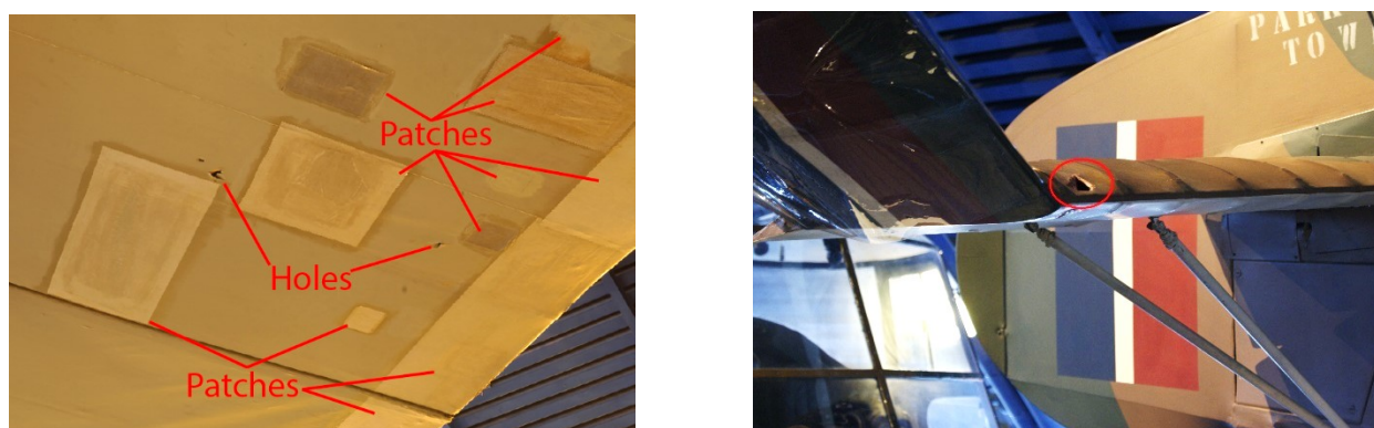
Figure 3-2: Holes in the Vickers Vimy lower starboard wing (left) and Cierva C30a (right) potentially the result of human action
