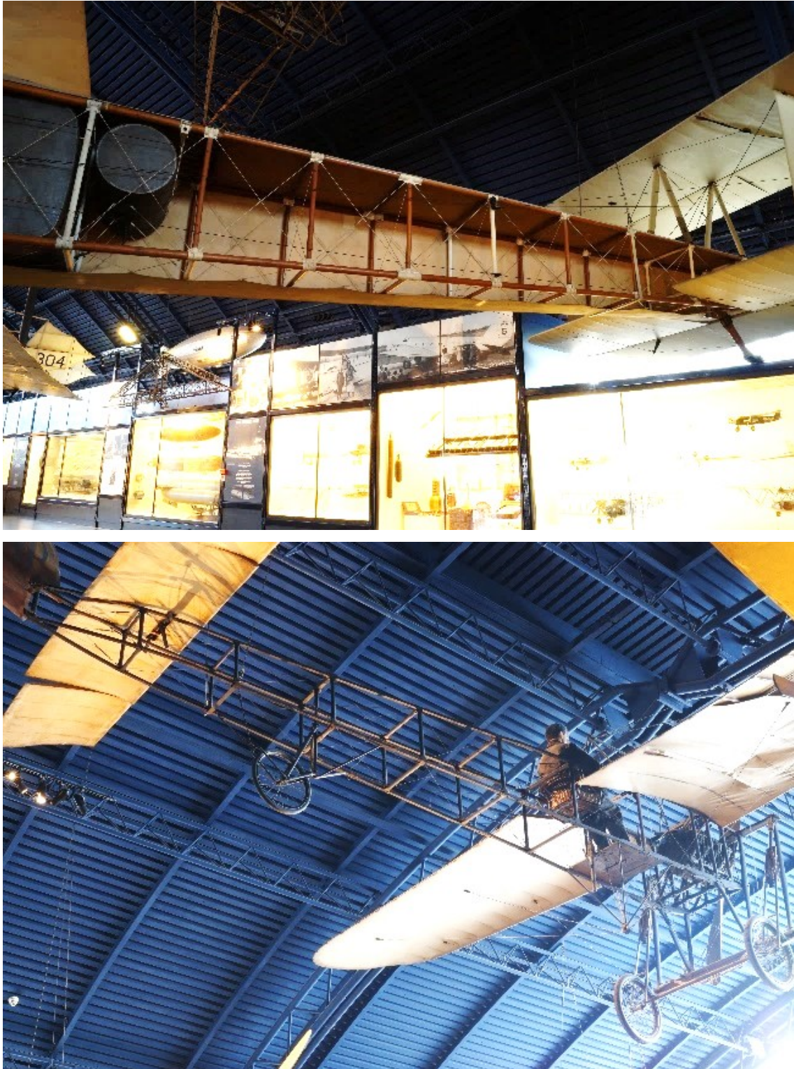
Figure 2-2: Aircraft fuselages on display in Flight made using the truss method. The Vickers Vimy is shown above, the JAP Harding Monoplane below
