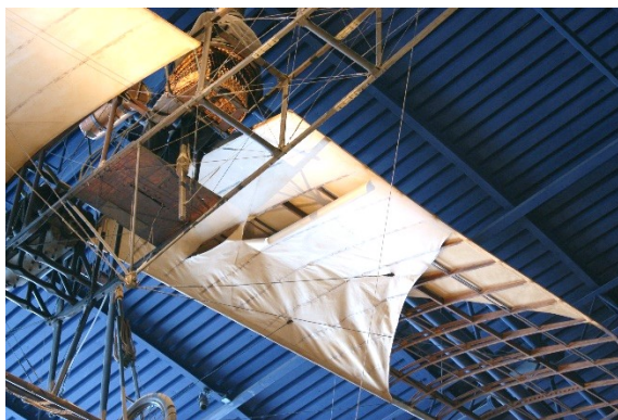
Figure 3-5: Tears in the doped-fabric skins of the JAP Harding Monoplane (left) and the Pterodactyl (right) lying well beyond human interference
