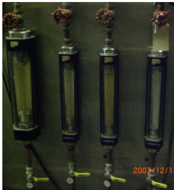
Figure 4.4. Photograph of the rotameters on LOTUS.
