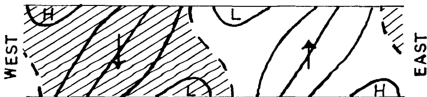
Fig 2.12 Vertical section along a line of latitude of the Eady decaying solution with isopleths of \psi (—), warm air ( shaded ) and vertical velocities ( arrows ).
