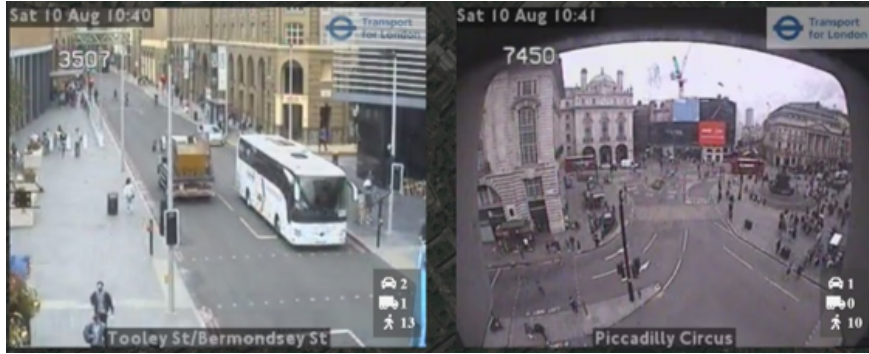
Figure 4: Two JamCam images with the (cars, trucks & pedestrian) counter overlay in their bottom-right corners.
