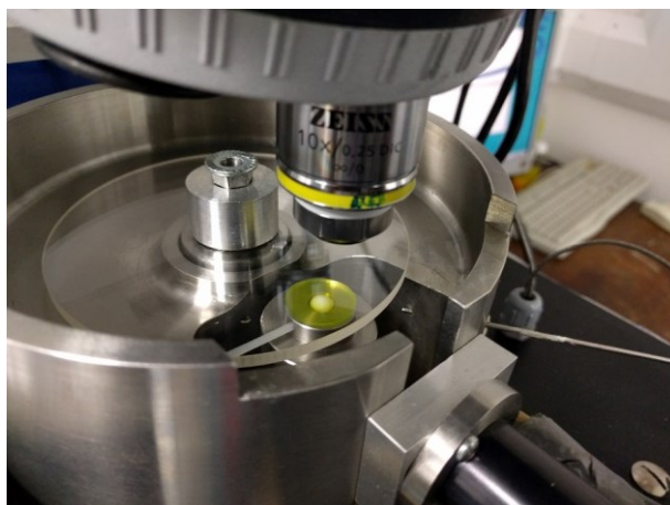
Figure 3.9: Test set up for dye interaction tests showing a transparent sapphire disc loaded against a PTFE ball submerged in 1mM CF mixed deionized water.
