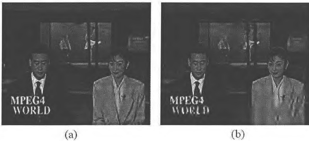
Figure 2.4: (a) Compressed image with uniform resolution scalable coding; (b) Compressed image with FSVC [WLB03]
