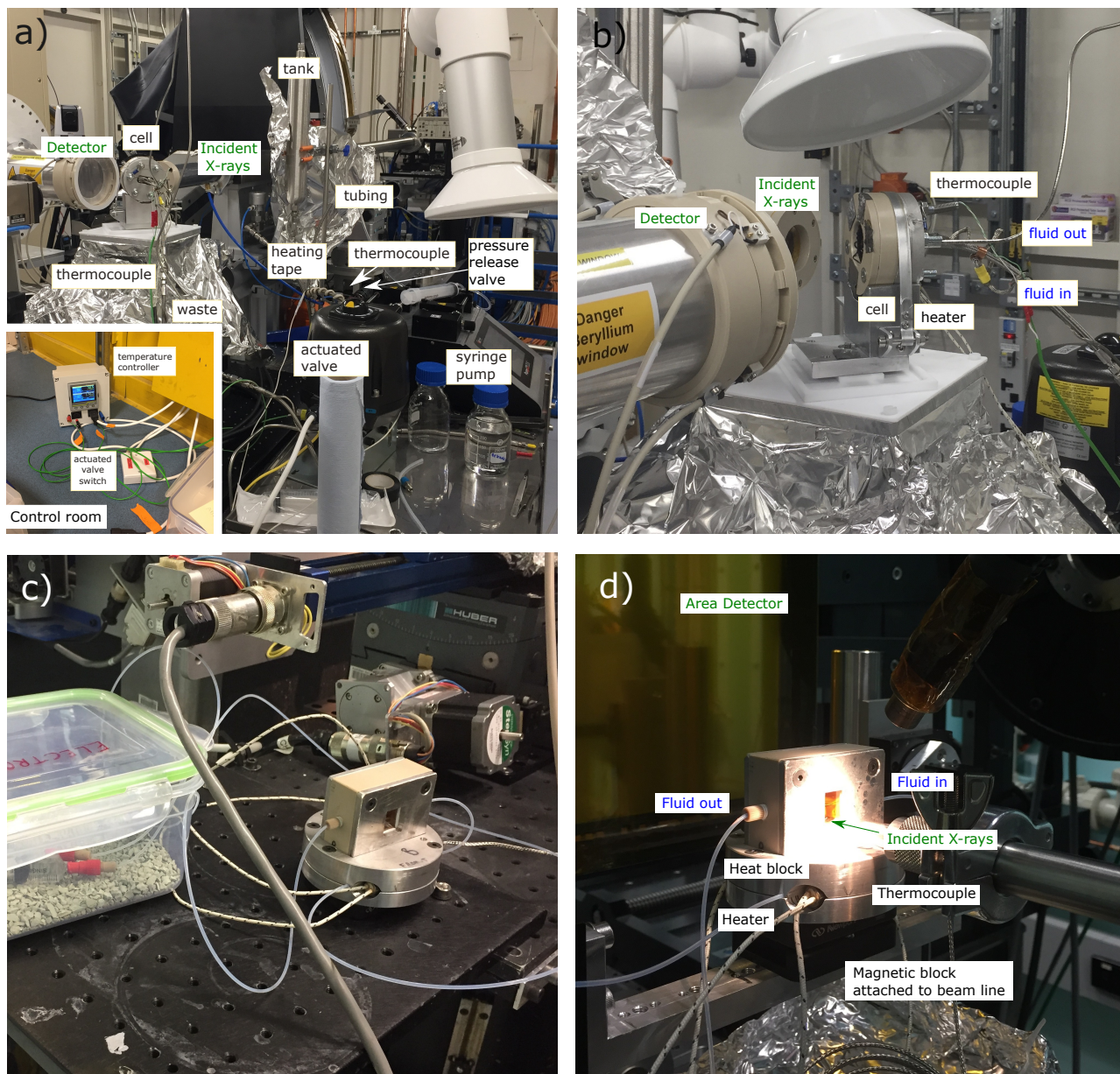
Figure 2.5: Photographs of the a) rig and b) cell on the I20 beam line at the Diamond Light Source. Images of the c) cell and d) beam line set up for measurements completed on the SAXS/WAXS beam line at the Australian Synchrotron.
