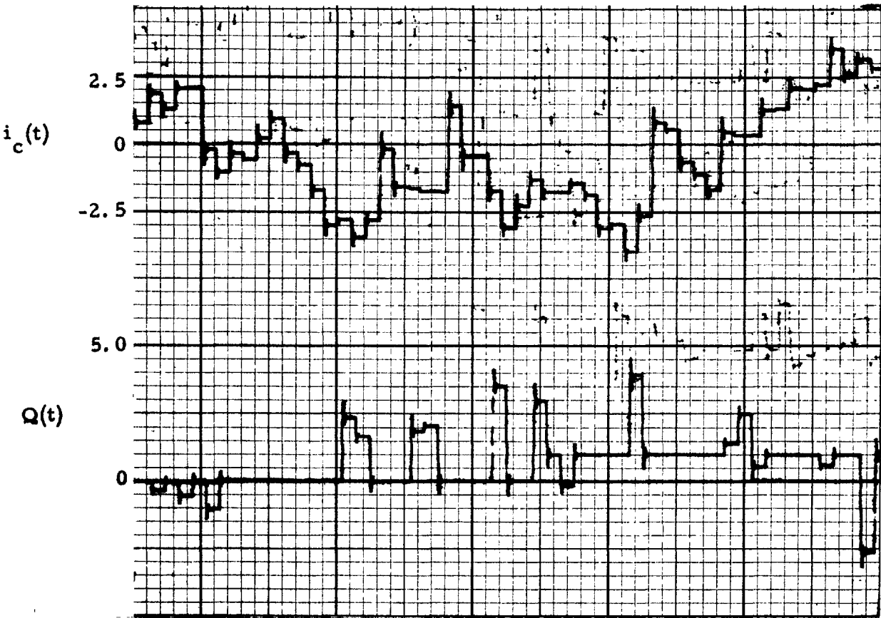
FIG 4.43 NON LINEAR SYSTEM RESPONSE TO A STEP PLUS NOISE
