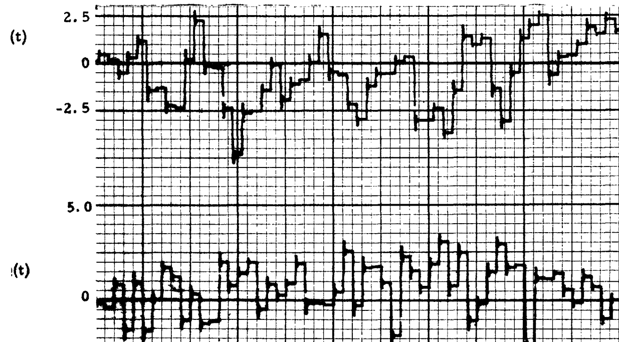
FIG 4.44 LINEAR SYSTEM RESPONSE TO A STEP PLUS NOISE
