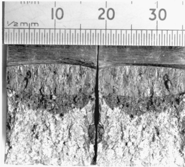
PLATE 5.1a Titanium alloy (6Al-2Cb-1Ta-1Mo) crack face, fatigue precracked with constant \Delta K or K_{max} .
