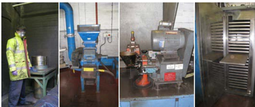
Figure 10: Equipment used for fuel preparation in the Central Support Laboratories of RWE. From the left: 50 cm sieves for grading; hammer mill; 11" disc mill; fuel drying oven.
