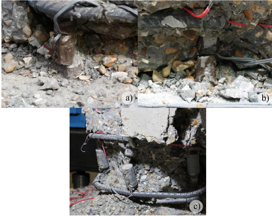
Figure 9 a) Reinforcement fracture mode for C300-C0-N0 and C300-CC-N0, b) reinforcement fracture in C300-CS-N0, c) fracture at the couplers-to-rebar interface in C300-CC-N1 following buckling of reinforcement
