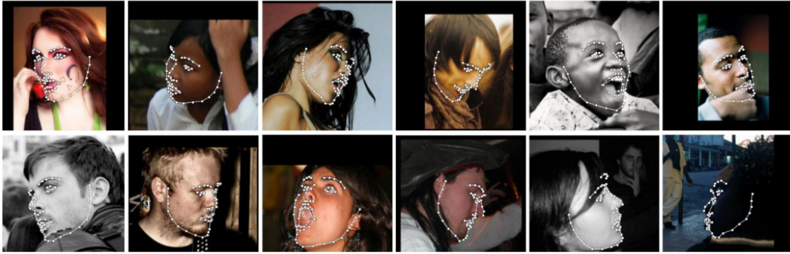
Figure 2.5: 68-point landmark estimation examples using a 2D-FAN. Source: https://github.com/1adrianb/face-alignment
