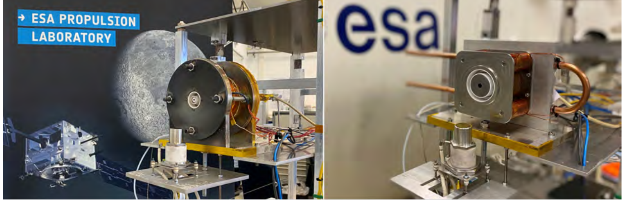
Fig. 1 Hall Effect Thrusters at the ESA Propulsion Laboratory of the European Space Agency. Left: Thruster WET-HET and cathode Hydrocat . Right: Thruster AQUAHET and the cathode Hydrocat . These devices are mounted on the Imperial Plasma Propulsion Laboratory thrust balance.
