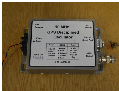
Figure 3.4: GPS module used for array synchronisation.
