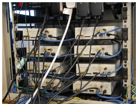
Figure 4.4: Multi-USRP hardware configuration for the 8-element UCA, USRP boards share a common clock that is generated by a GPS module.
