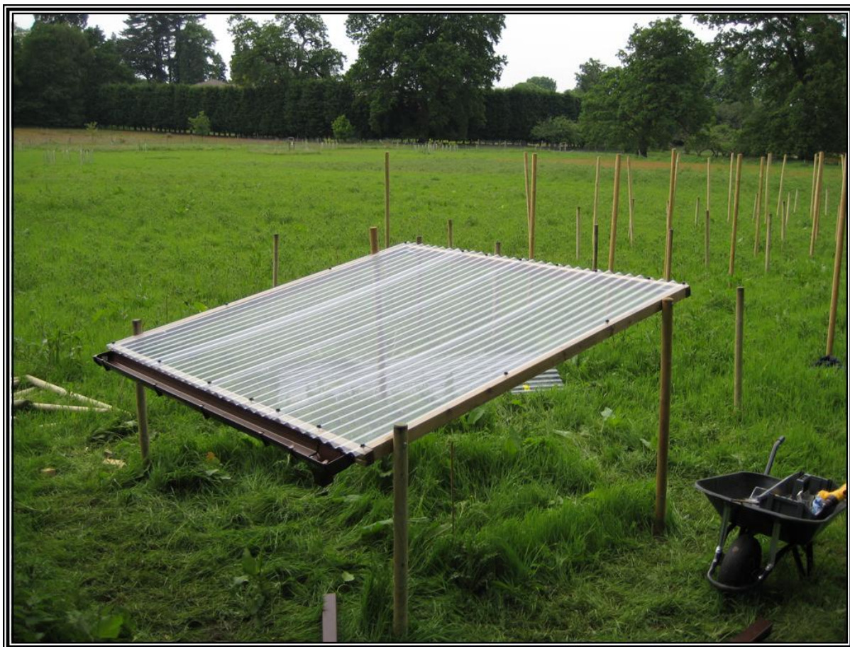
Figure 1: Initial stages of the DIRECT experiment, showing the prototype with corrugated plastic, circa May 2008.
