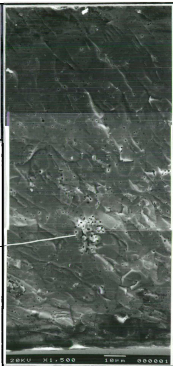
Figure (4.10) - transgranular fracture path and porosity distributed throughout fracture face of set B, and sometimes in clusters.
