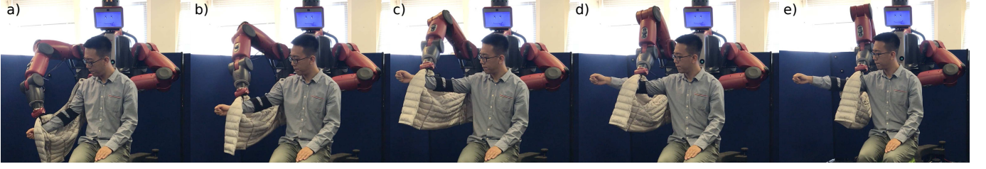
Fig. 3: Snapshots of the robot-assisted dressing sequence from a user with simulated elbow movement limitations. (a) The robot reaches the initial hand position and starts the dressing trajectory. (b) The user moves his arm suddenly. (c) The robot adapts its motion accordingly and updates its trajectory in real time. (d) The robot reaches the updated elbow position. (e) The robot finishes dressing the right arm.
