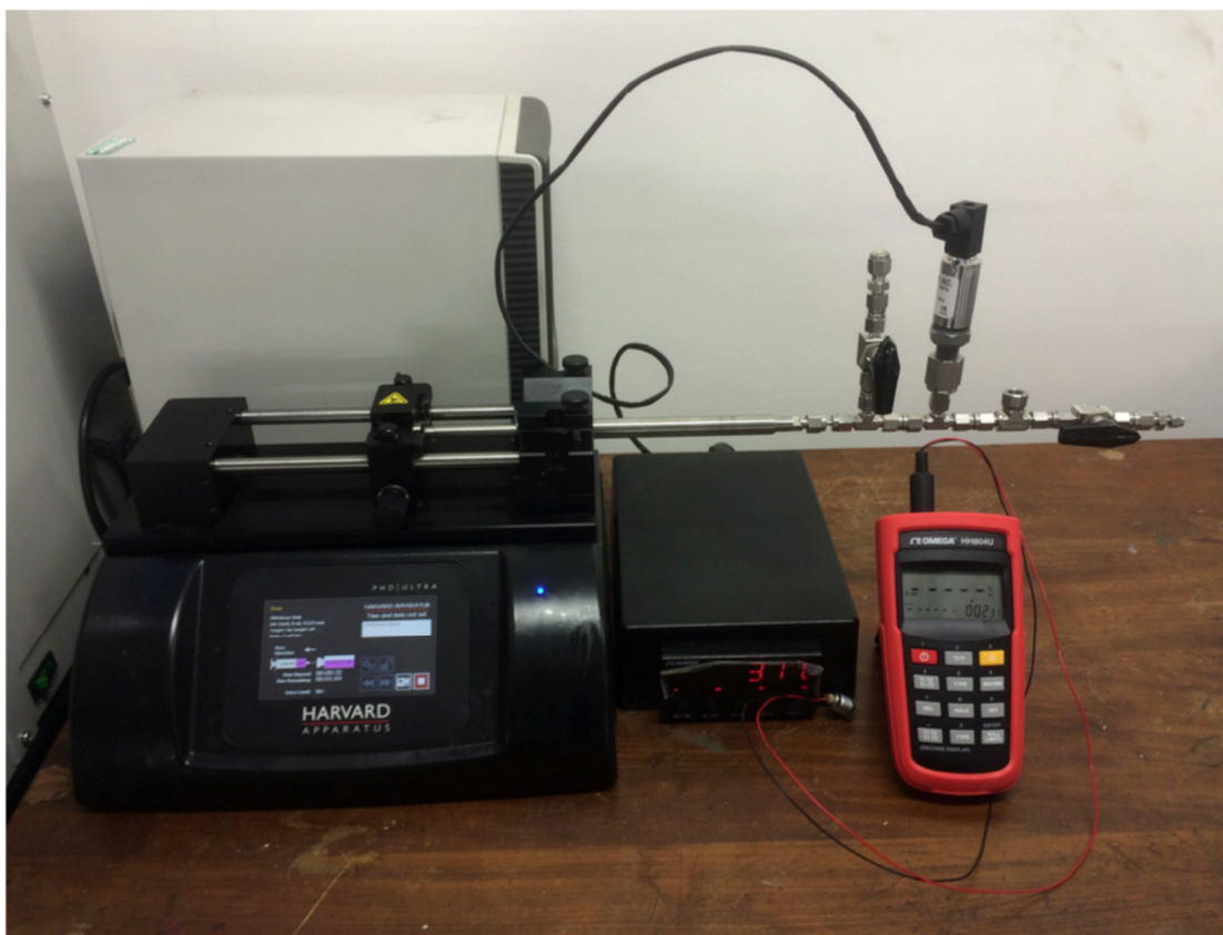
Fig. 10.3: Pressure syringe viscometer
