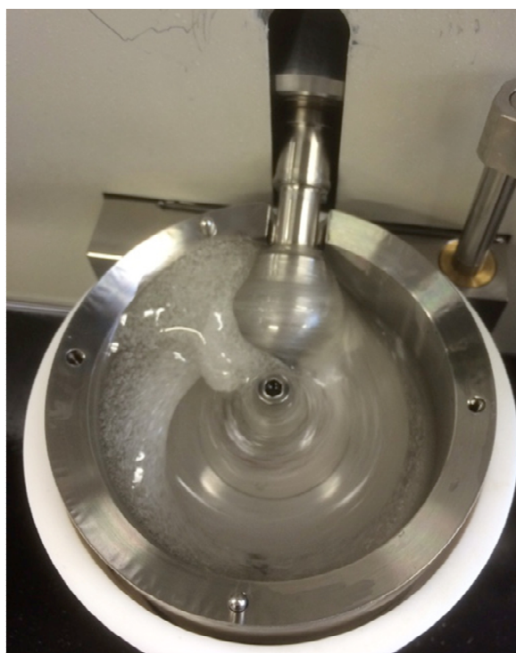
Fig. 6.1: PMMA disc, steel ball MTM test implementing a very thick oil
