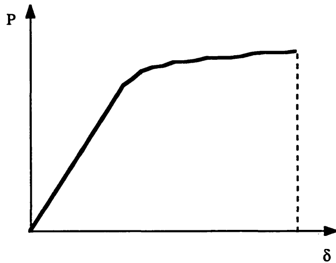
Figure 2.4.1: Typical tensile load-displacement curve for ductile fracture.
