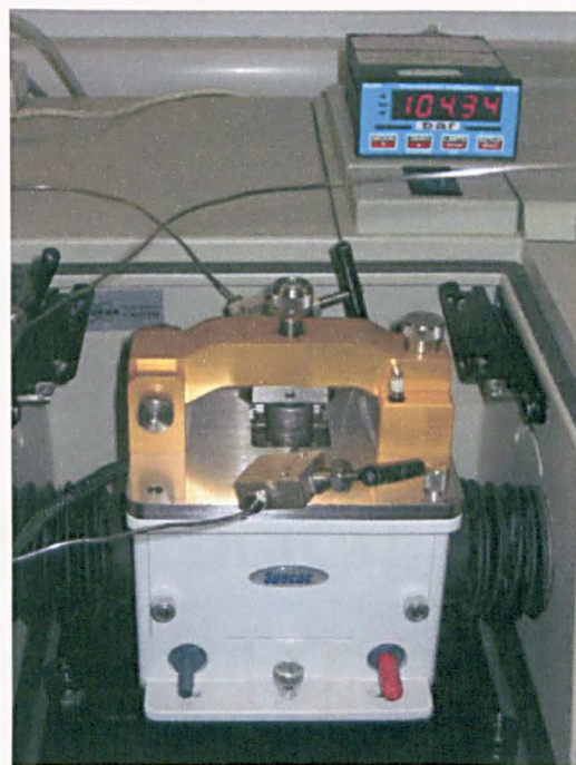
Figure 5.3. ATR FTIR in situ high-pressure rig assembly shown schematically (left) and a photograph showing the high-pressure cell in position on the Golden Gate TM accessory (right).
