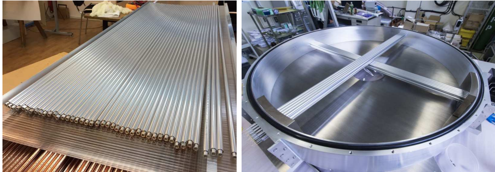
(a) Straw Tube Construction and Prototype Tracker
