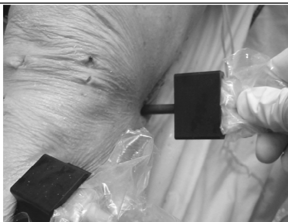
Figure 3.6: the digitising sensor instrumented on a calibrated stylus
