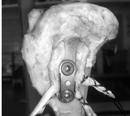
Figure 11.6: new DB hamstrings fixation device consisting of a plate and two bicortical screws.
