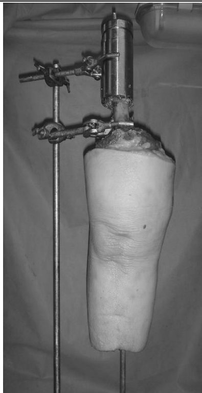
Figure 3.1: a knee potted in the vertical position to minimise varus-valgus moment
