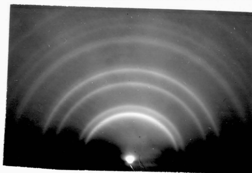
Fig.53. 27,000 Å Ni at 460 mA/cm 2 on polished polycrystalline Cu, stirred bath, 50°C.
