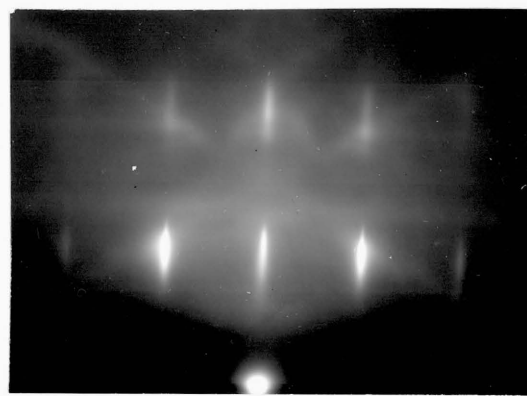
Fig.81. 25,500 Å Ni at 500 mA/cm 2 on Cu (110), stirred bath, 50°C.
