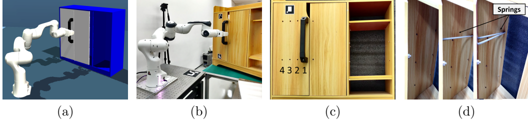
Figure 5.2: (a) and (b) show the hardware setup in the real world and in simulation. The Aruco markers attached to the table and the cabinet are used for tracking purposes. (c) shows four different locations of the doorknob, each separated by 5\text{cm} along the lever arm of the door. (d) shows three variants of the door. From left to right are the original door, the door with one spring and the door with two springs attached to the hinge. The springs were used to emulate doors with different dynamics.
