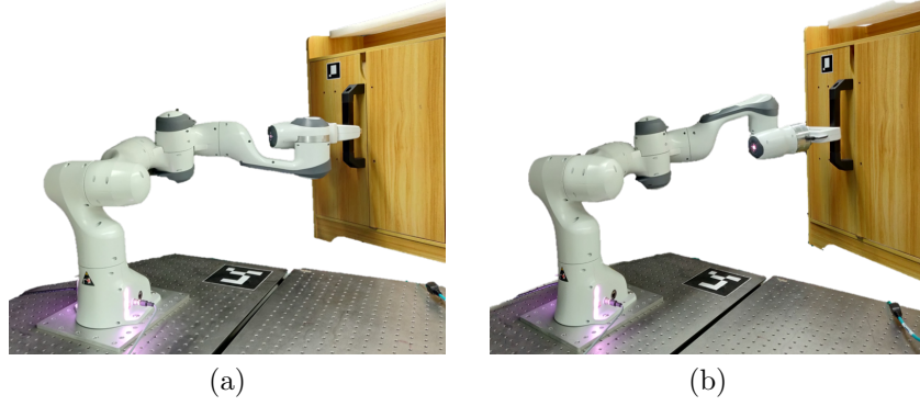
Figure 5.3: Two different initial robot poses were used in the human demonstration. (a) is the initial robot pose used to estimate parameter distribution in Tab. 5.1. (b) is another initial robot pose used to validate the possibility of a bias in parameter estimation.
