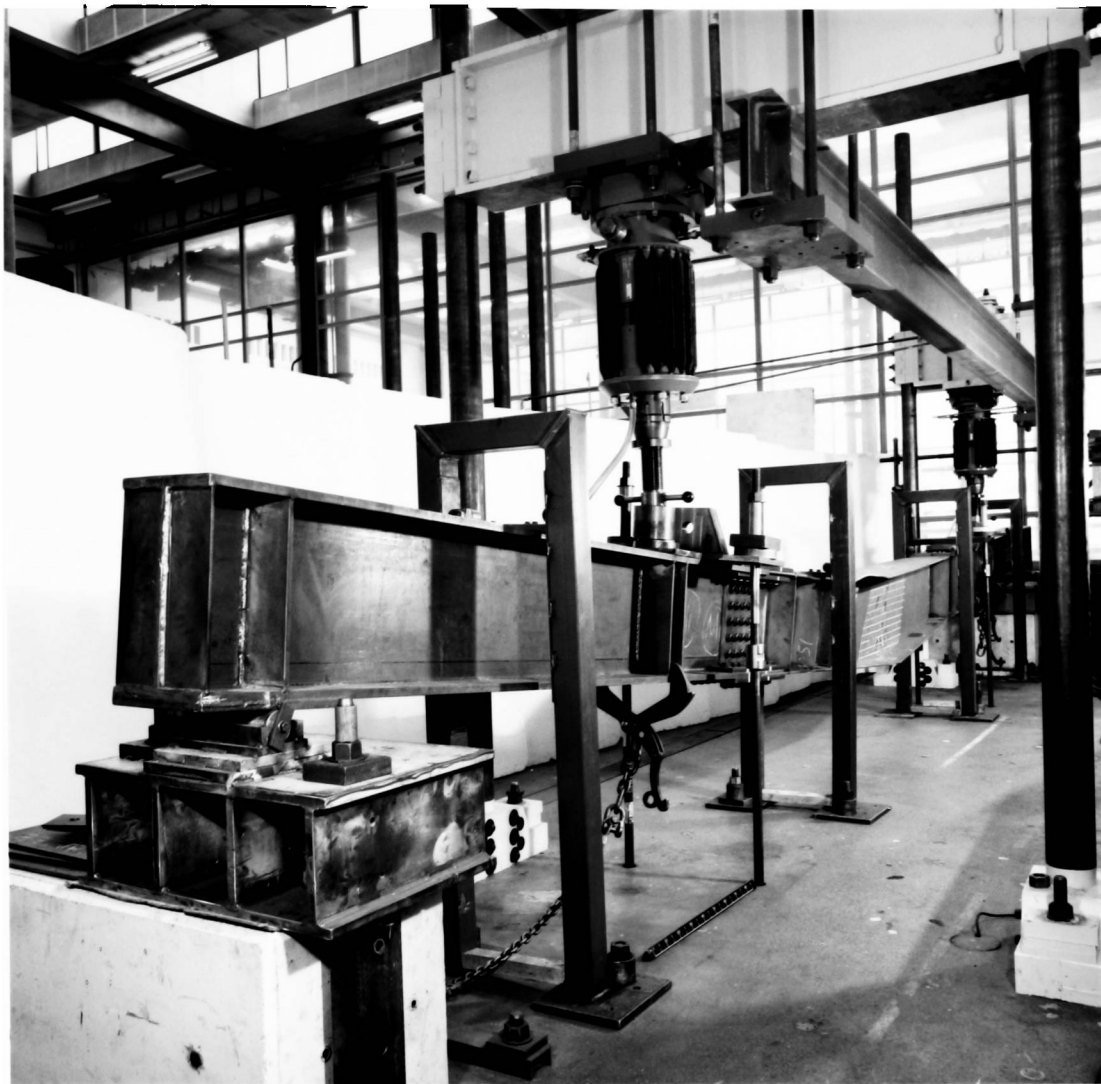
Plate 20 - Failure of Beam 5 ( t_{fc} = 15\text{mm} ).
