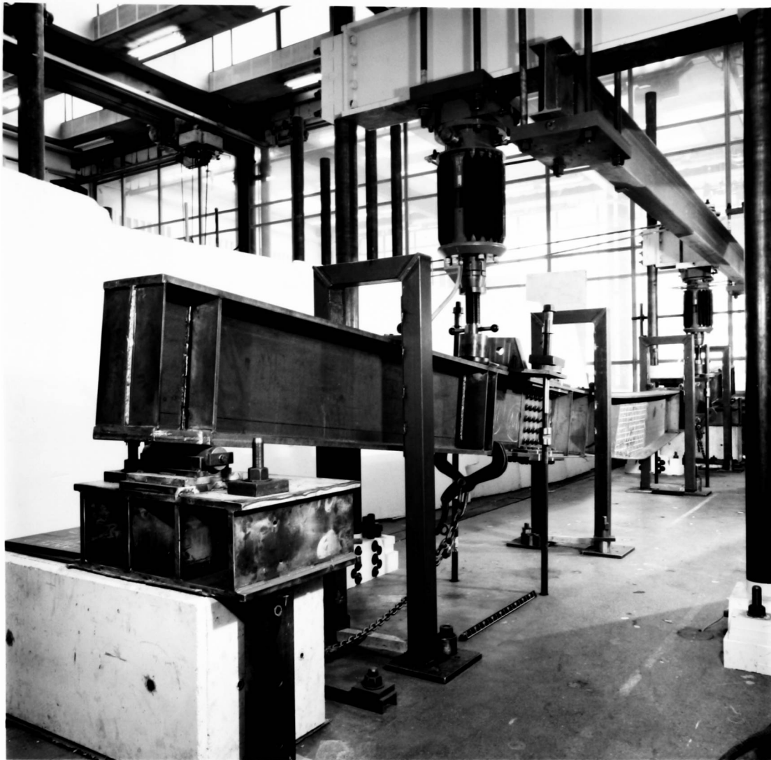
Plate 18 - Failure of Beam 4 ( t_{fc} = 20\text{mm} ).
