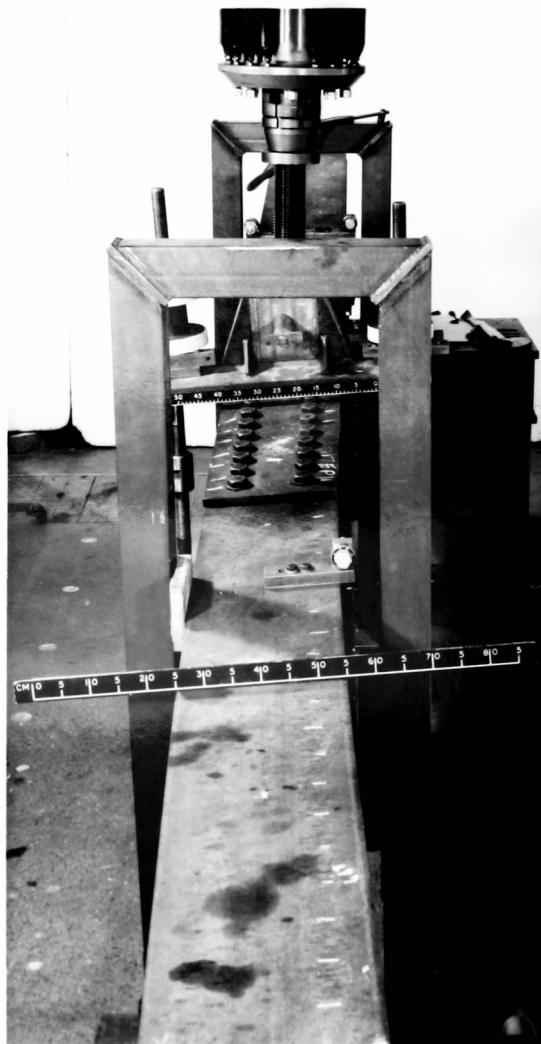
Plate 8 - Detail of the failure of Beam 1 ( t_w = 7\text{mm} ).
