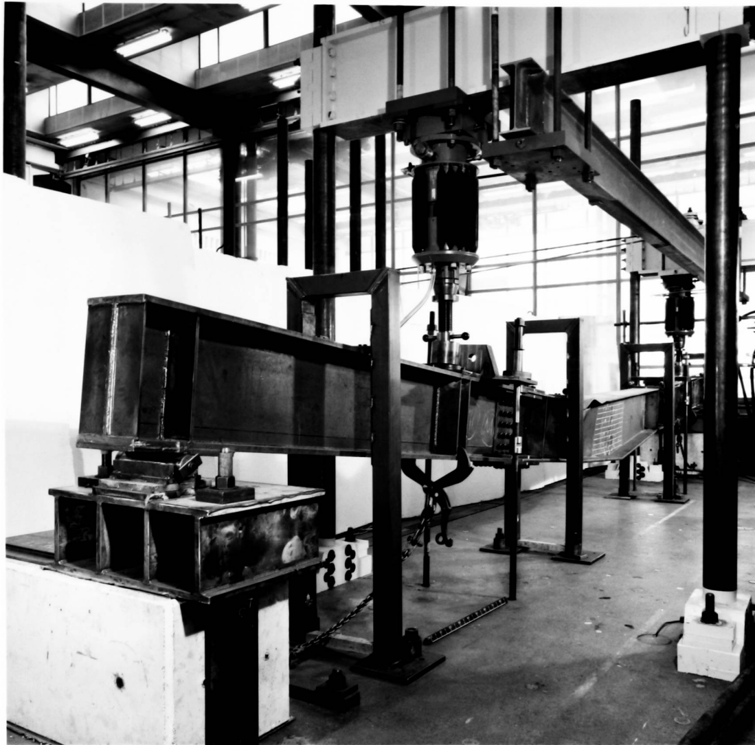
Plate 22 - Failure of Beam 6 ( t_f = 25\text{mm} ).
