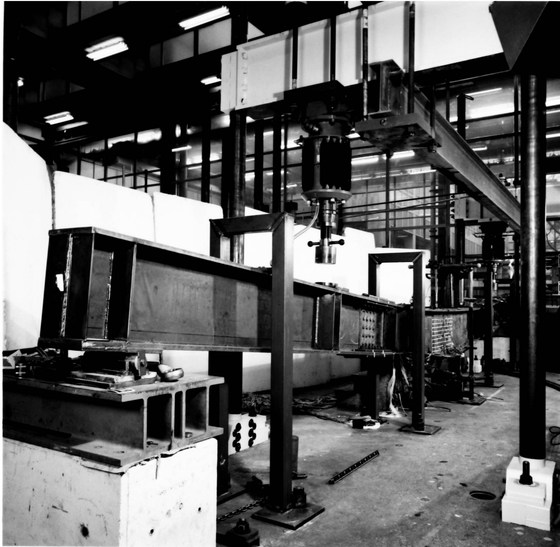
Plate 7 - Failure of Beam 1 ( t_w = 7\text{mm} ).
