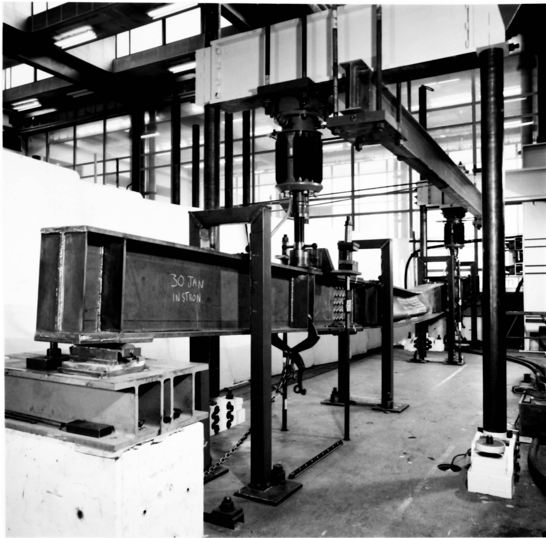
Plate 11 - Failure of Beam 3 ( t_w = 3\text{mm} ).
