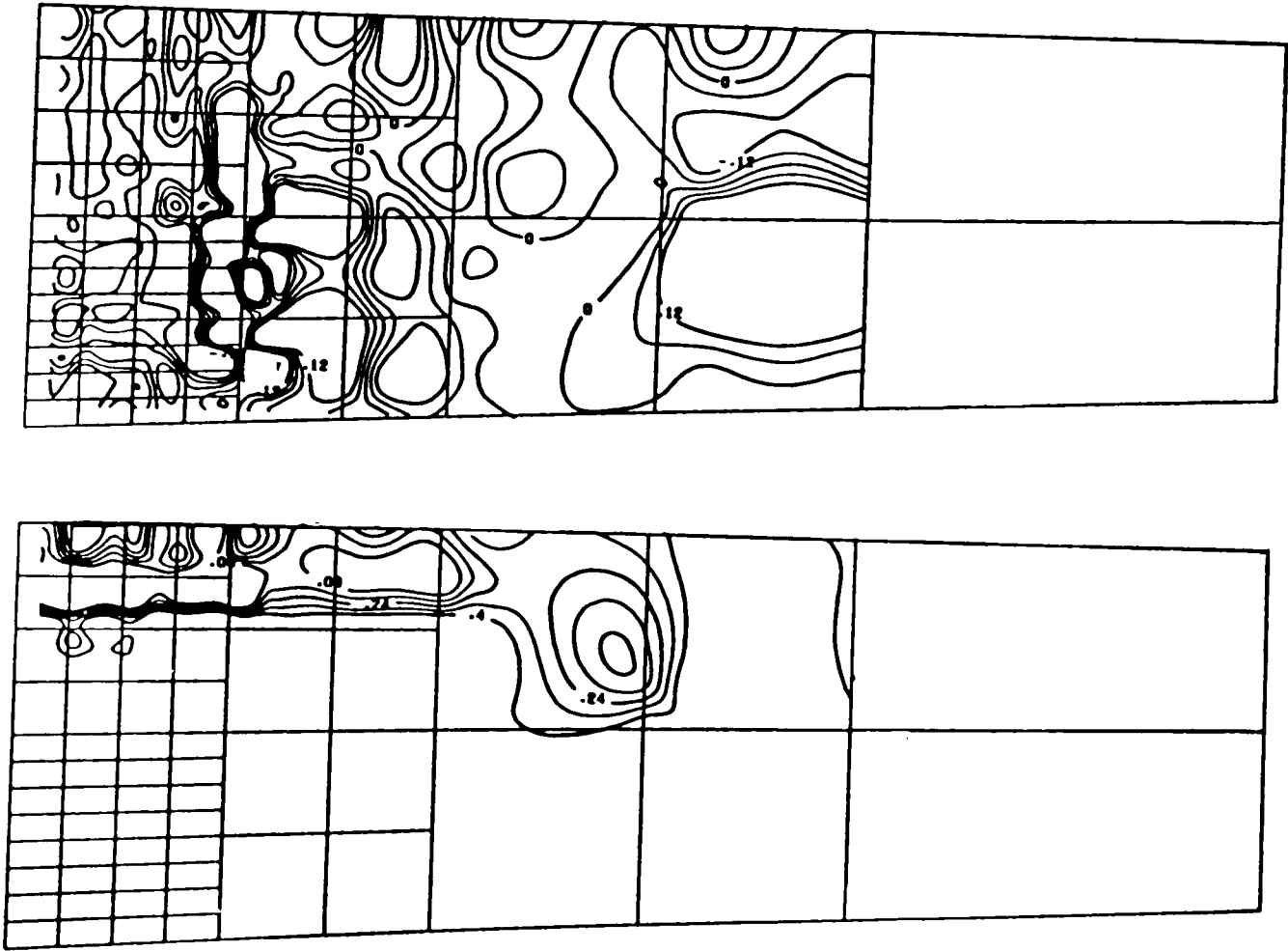
Figure 5.49 - Deformed Configuration of the Beam with \alpha = 2.86^\circ ( t_w = 5\text{mm} ).
