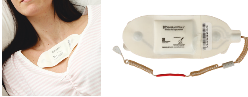
Figure 1-4: A test subject wearing the state-of-the-art electrical impedance pneumography based respiratory monitoring system (Sensium Healthcare SensiumVitals®) and close-up photo of their patch sensor [102].
