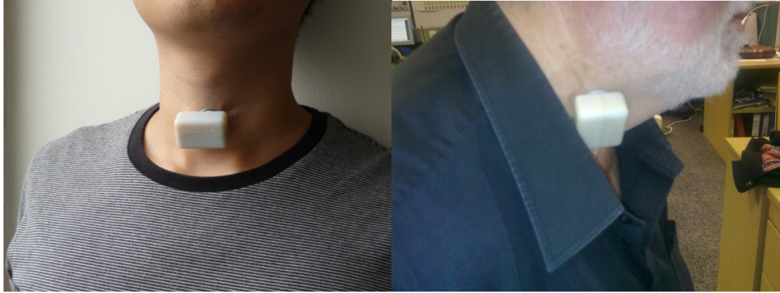
Figure 6-1: Wearable respiratory activity monitor worn by myself [155] and a volunteer.
