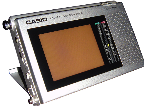
Figure 1.2: A Casio TV-10, the world’s first commercially available LCD, TFT-based display, released in 1983.
