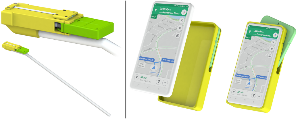
Fig. 3. Conceptual illustrations of future integrations of the S-BAN concept with (left) a guide cane for VI users and (right) a smartphone case. Both devices use shape to haptically communicate spatial guidance commands without reliance on sight or sound.
