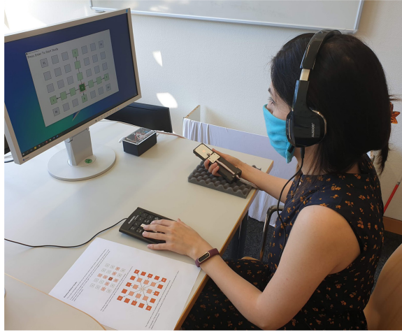
Fig. 7. Arrangement of the perceptual study. Participants held the S-BAN in their dominant hand and entered pose choices via a cursor controlled by a numeric pad. This image shows a training phase. In the actual experiment, the user's dominant hand and S-BAN are covered with an opaque box.
