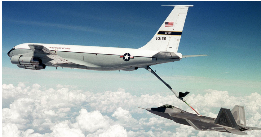
Figure 2.4: KC-135E performs an air refueling operation on F-22A [14]
