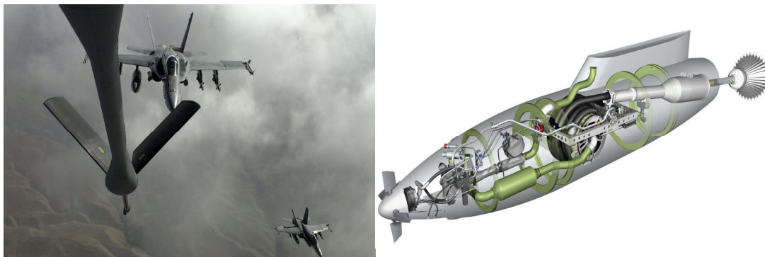
Figure 2.6: Telescopic boom (left) [14] and wing pod layout (right) [75]
