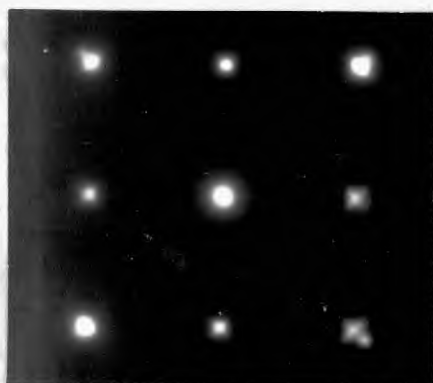
(B) A CdS layer deposited at 10 Å/sec. on a vacuum-cleaved NaCl(100) substrate at 200°C.
