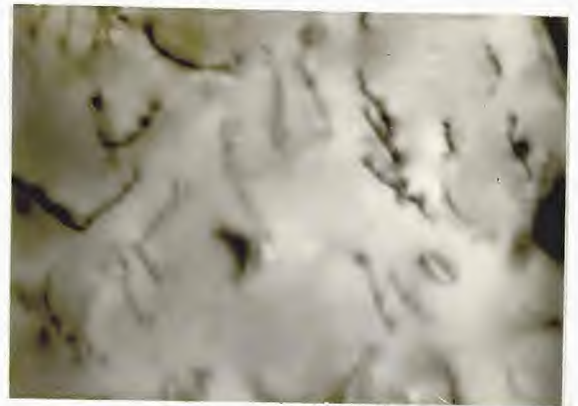
(B) SUBSTRATE TEMPERATURE = 200^{\circ}\text{C} . \overline{0.1\mu}
