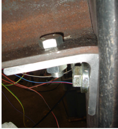
Figure 3.12: Column face deformation in the compression zone of Specimen B10-G8.8-d40-M.
