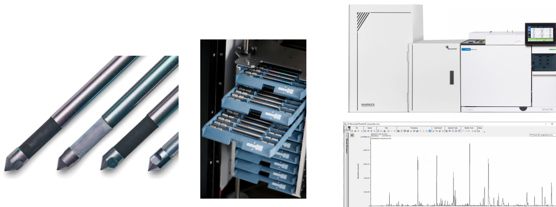
Figure 46. High capacity sorptive extraction-thermal desorption method for static headspace extraction (Images from Markes International)
