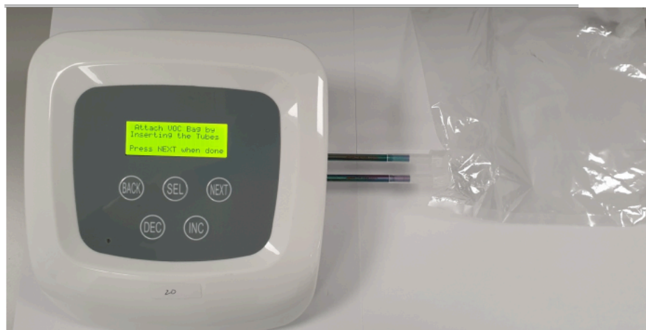
Figure 23. Correct setup of the breath collection bag, TD tubes and gas sampling pump
