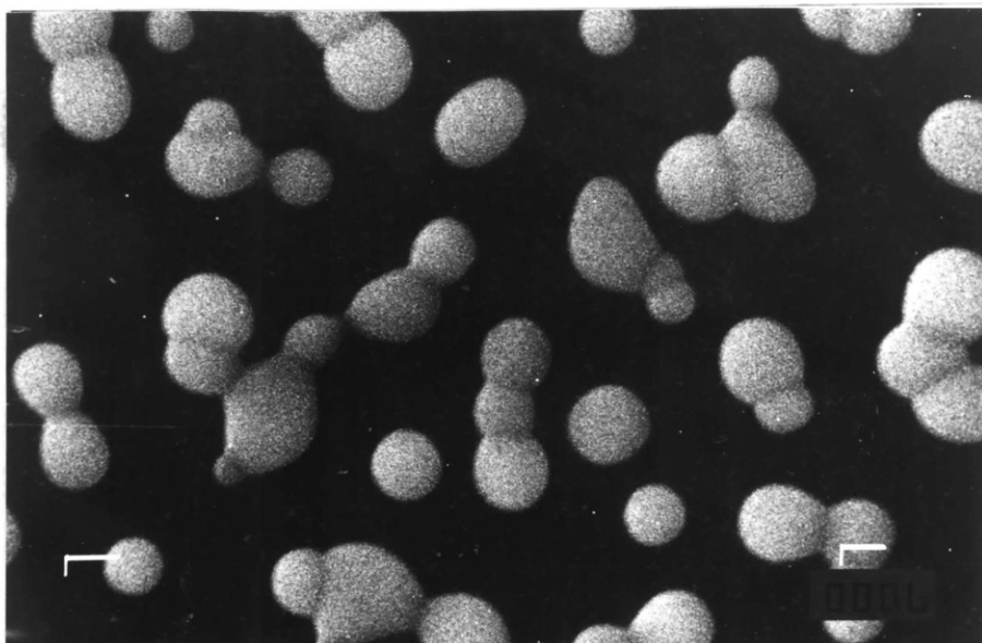
Fig. 7.5. CsCl film structure after exposure to laboratory air for several minutes (average thickness 6800 Å (Talystep)). Substrate Si (1400 Å SiO 2 ), Rate ~ 340 Å/min.
