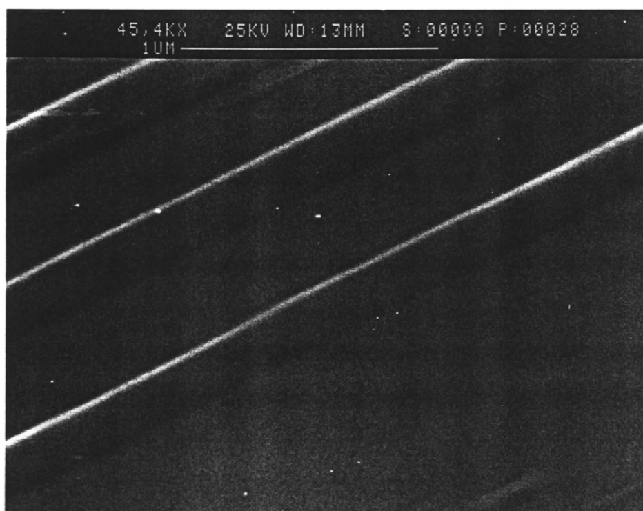
Fig. 6.28. Linewidth of 0.38\ \mu\text{m} obtained with the group 1f lines.
