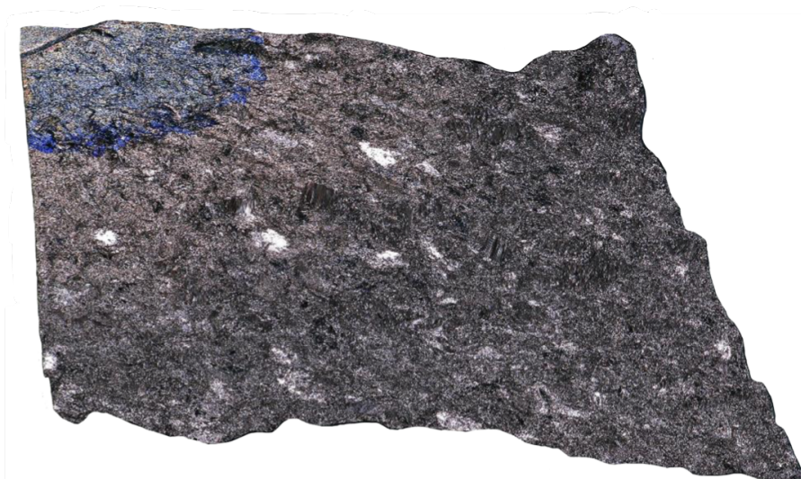
Figure 8.8: Tilted view of the fracture surface in Figures 8.3 and 8.7. It can be observed that at larger crack length shiny flat regions are observed and pull out of whole colonies, whereas cleavage of the colonies is observed as shorter crack lengths.
