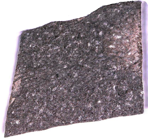
Figure 6.7: Optical micrograph of 0.06 mm notched naturally initiating specimen, 5 x 5 mm fracture surface from an angle showing the surface topography. Image taken using Keyence VHX-5000 at Rolls-Royce plc. Bristol, courtesy of Edward Saunders.
