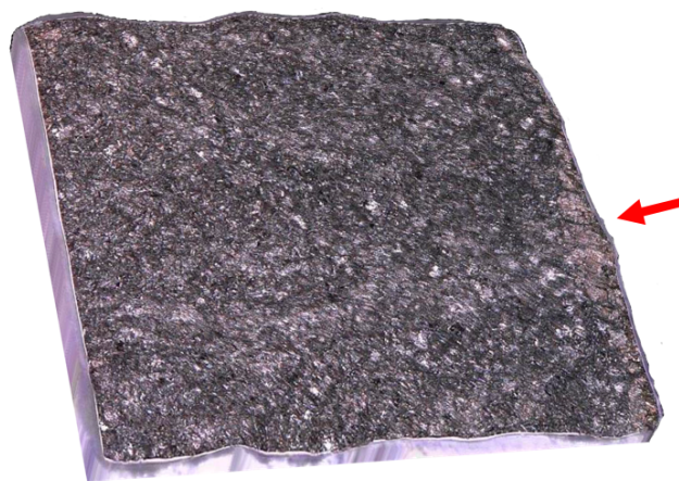
Figure 6.12: Optical micrograph of 0.03 mm notched naturally initiating specimen, 5 x 5 mm fracture surface from an angle showing the surface topography, with a red arrow indicating the region of fatigue. Image taken using Keyence VHX-5000 at Rolls-Royce plc. Bristol, courtesy of Edward Saunders.
