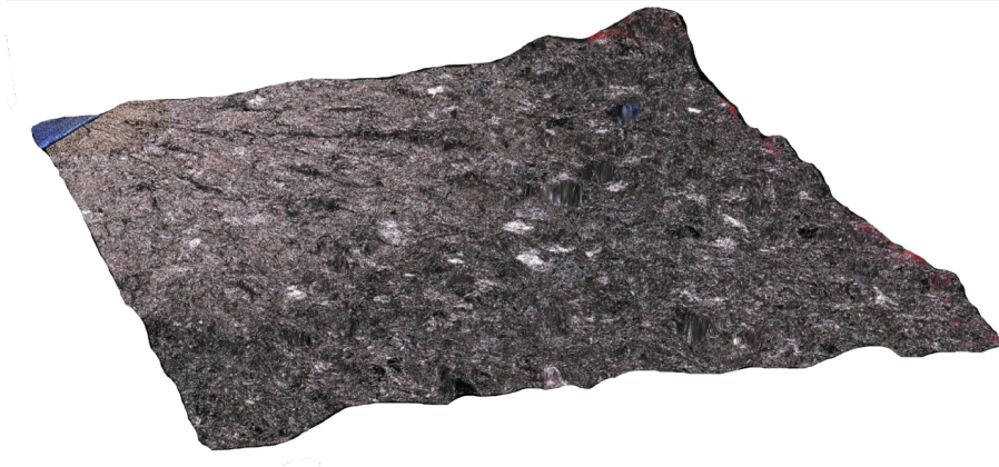
Figure 8.12: Fracture surface at a tilt of the application of a compressive load during crack growth.
