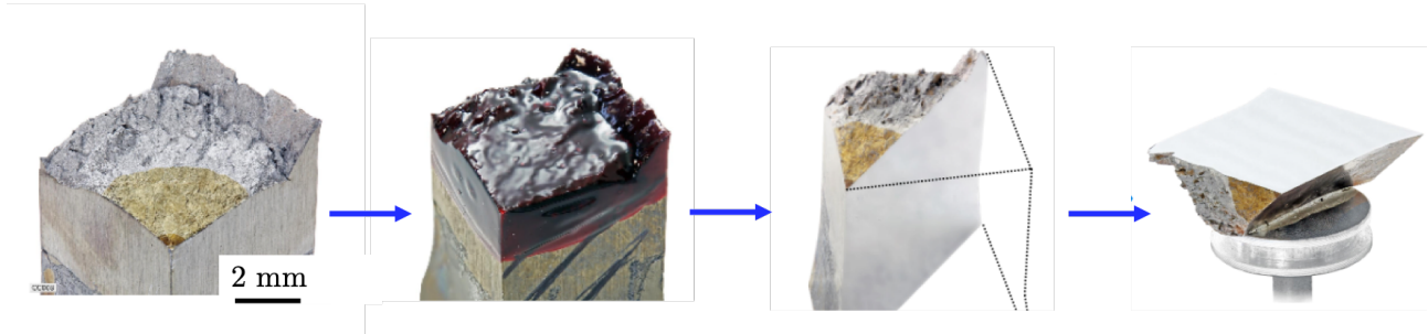
Figure 3.4: Fracture surfaces were dipped in Microstop and left to dry before being sectioned and polished. The Microstop was then removed and the sample fixed to a stub for microscopy. Images courtesy of Tom Zalewski, Rolls-Royce plc..
