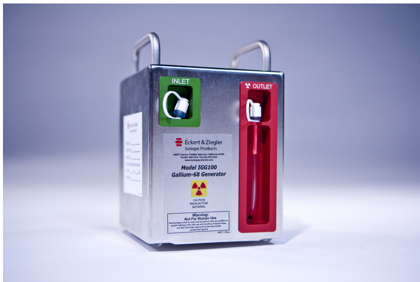
Figure 4.1: Eckert & Ziegler Model IGG100 Gallium-68 Generator, similar to the one used in this project. Picture taken from www.radiustech.it . 3
