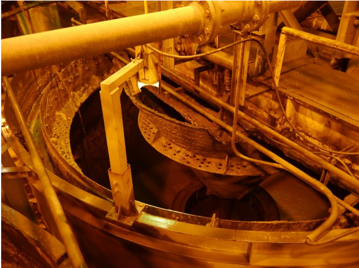
Figure 2.12 - Conical crowder in an Outotec flotation cell (own photograph).
