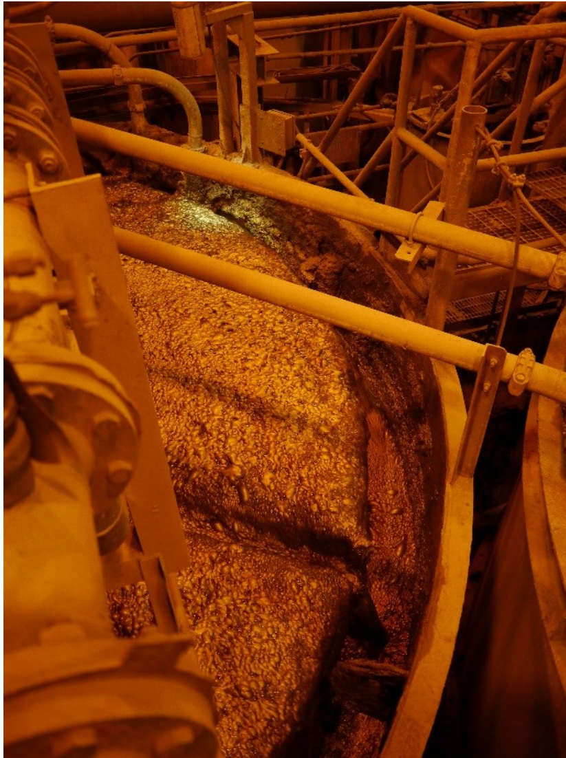
Figure 2.11 - Radial launder in an Outotec flotation cell (own photograph).
