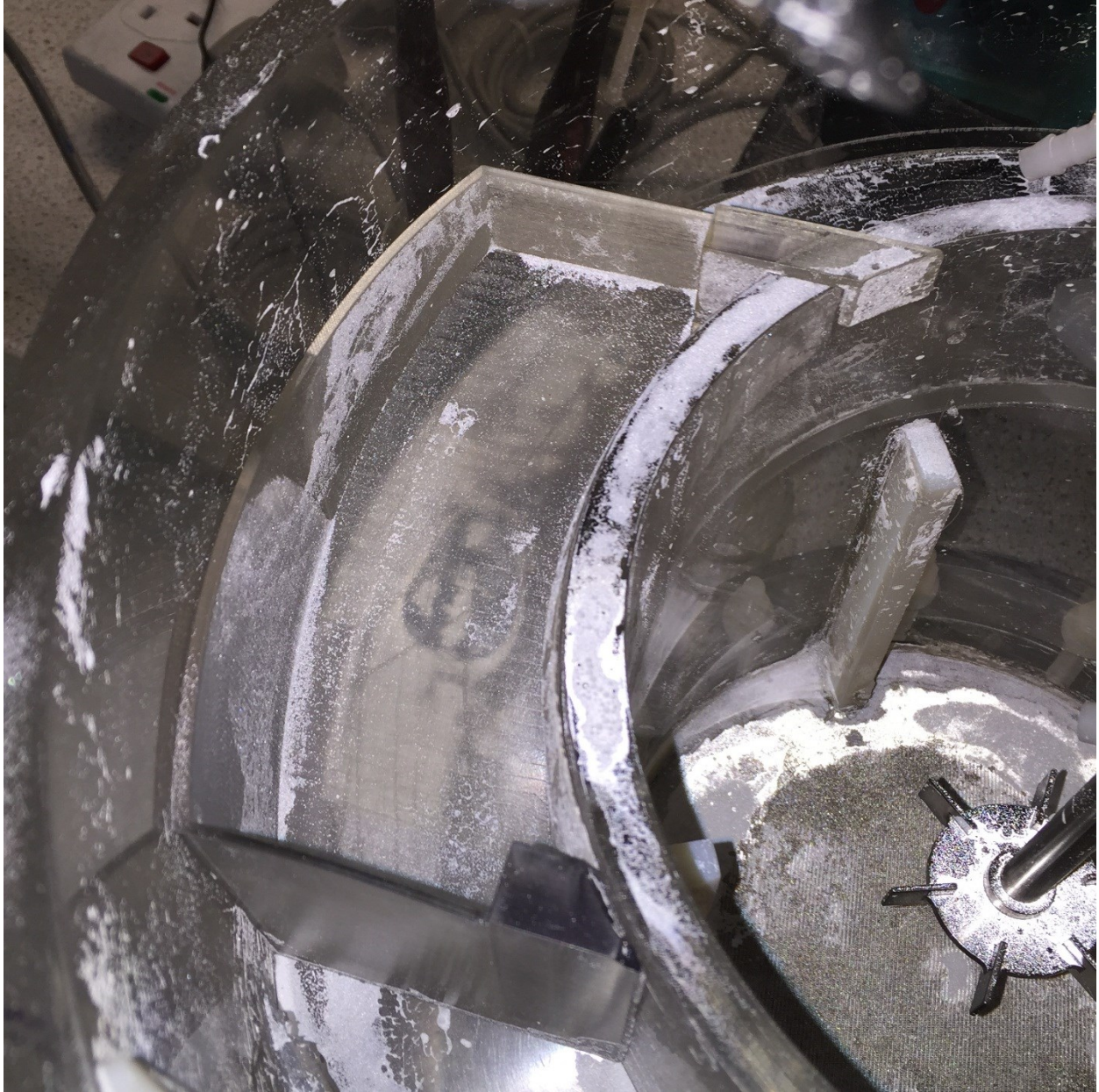
Figure 3.10 - 3D printed scoop sitting inside the flotation cell launder
