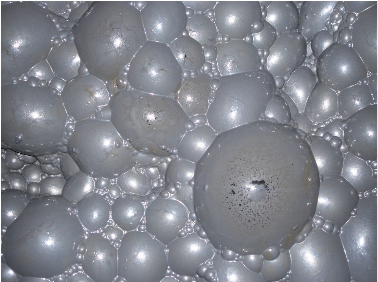
Figure 2.4 - Zinc flotation froth, Lisheen, Ireland (research group photograph).
