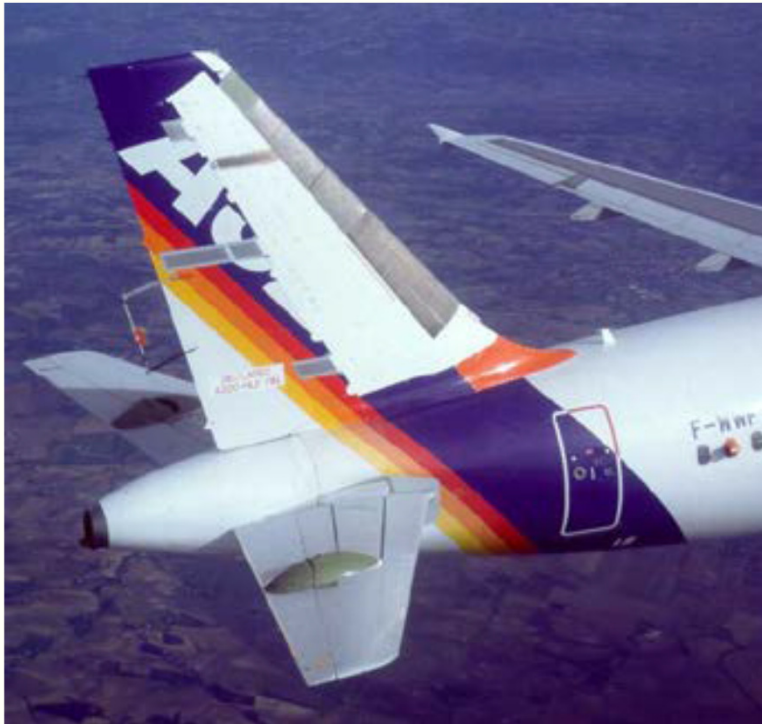
HLFC system on A320 fin
