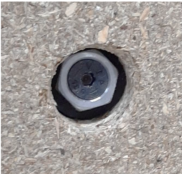
Fig. 18. Rotation and pull-through failure of specimen 2-P15-P3.
