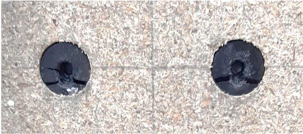
Fig. 17. Failure of specimens 2-P15-P1 and 2-P24-P1 showing the split fittings.
