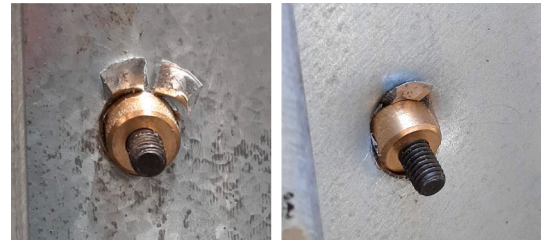
Fig. 20. Failure of the Type 4 connector - failure of the four locking segments followed by the bevelled nut pulling into the CFS sheet.
