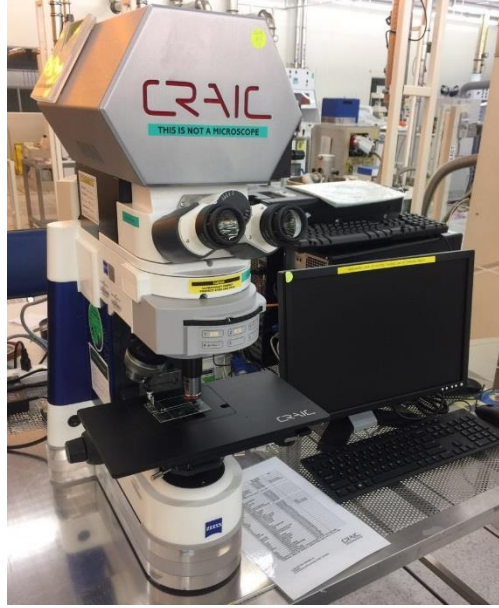
Figure 2.8 | Photo of the CRAIC UV-VIS-NIR micro-spectrophotometer (model QDI 2010) used to measure reflectance spectra.
